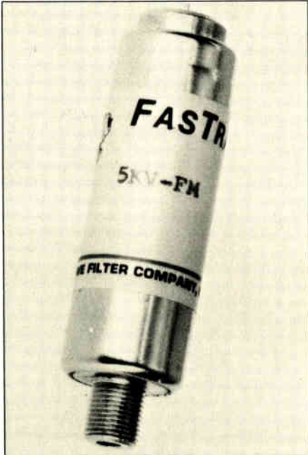
Typical Pay TV trap for VHF channel 23, retuned to suppress commercial mobile radio at 220 MHz—to remove overload to antenna pre-amps receiving VHF high band TV channels.
