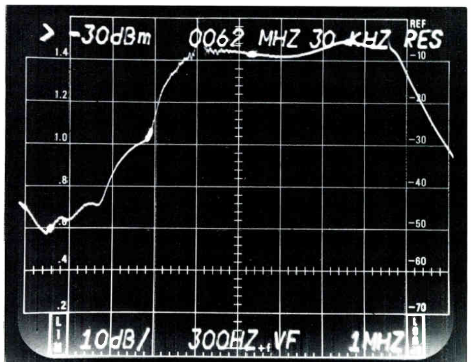
Figure 7-9 Swept modulator response using 1405. Markers are at 1.25 MHz, 3.58 MHz and 4.75 MHz
