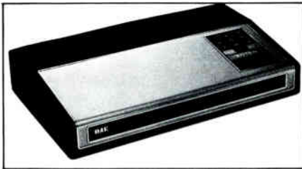
The Oak Moduline model KDM 400 56-channel synthesized converter/decoder.
