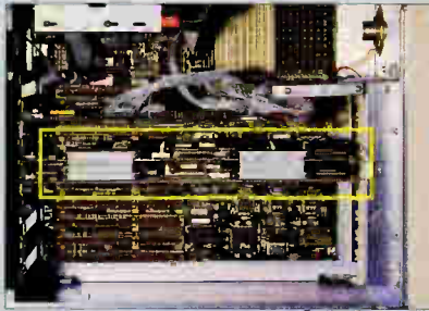
Each 486DX2 chip sits on a circuit card (outlined) in an extended EISA slot with a 512-KB RAM cache. The two CPUs communicate via two ribbon cables.
