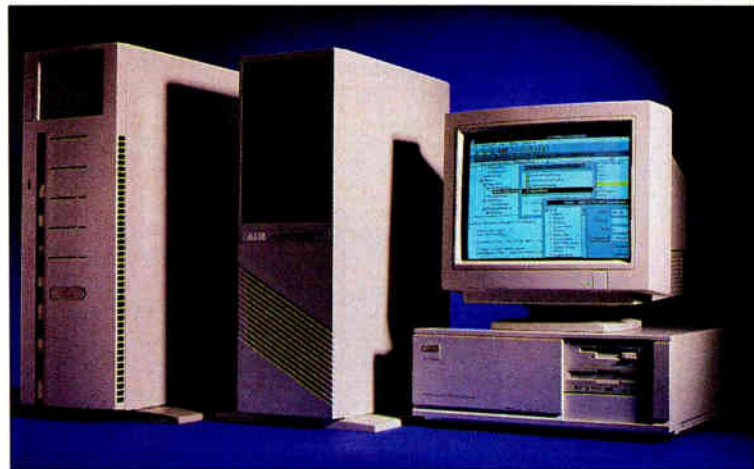
Three dual-processor systems from Compaq, ALR, and VTech (left to right). The ALR ProVEISA DMP and the VTech Platinum SMP systems each have two 486DX2/66 CPUs. The Compaq ProLiant 2000 can take two 50-MHz 486DX or two 66-MHz Pentium processors.
