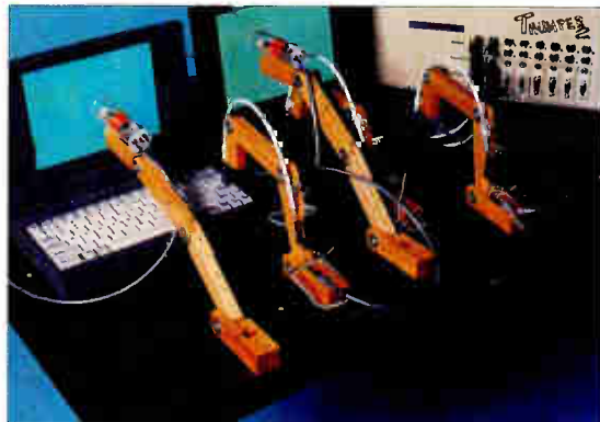
BYTE's Thumper 2 uses optical sensors to monitor power management in portables during battery-life testing.
