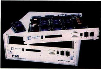
Zycad's Paradigm RP lets DSP developers test and simulate complex DSP designs prior to committing these designs to silicon.
