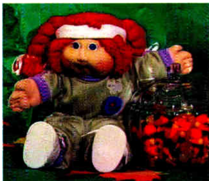
Photo 2: The Sony MVC-7000's resolution is lower than that of the Kodak camera, but its three CCD chips yield more accurate colors. Notice the slight pixelation in the doll's eyes. If you look closely at the blue button, you'll also see a bit of video bleed of the blue onto the gray background. The 768- by 493-pixel image printed at 300 dpi would be about 1.75 by 2.5 inches.
