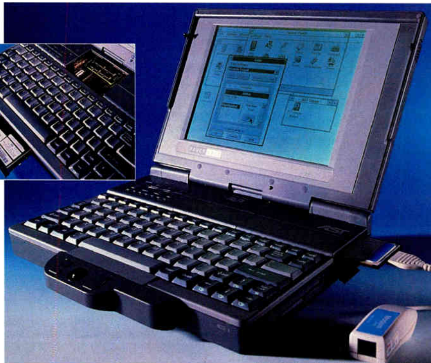
AST's new PowerExec notebook features PCMCIA support, a clip-on trackball, an upgradable screen, and (inset) a removable hard drive and an upgradable CPU.
