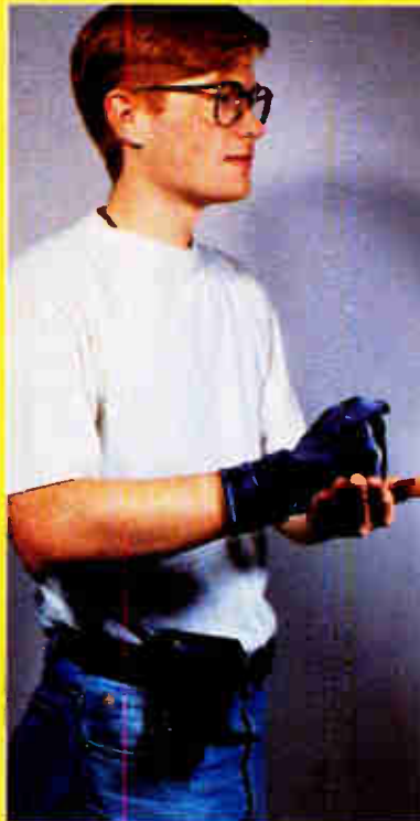
Photo B: To help hearing-impaired people communicate with those who don't use American Sign Language, students at Carnegie Mellon developed this prototype translator. The design uses gloves with sensors to send hand- and arm-movement information to a personal computer. Software converts the signals into English words, which are synthesized and output over a loudspeaker. (Courtesy of Carnegie Mellon University)
