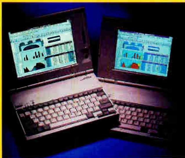
The Compaq LTE Lite 4/25C (right) uses Intel's new low-power 486SL processor. The LTE Lite/25E features an eye-grabbing active-matrix display.
