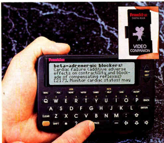
Digital books snap in and out at the base of the Digital Book System-1. You can cross-reference, highlight, and transfer text from one book to the other.
