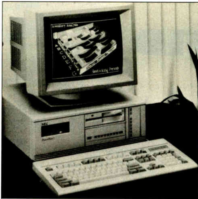
NEC's PowerMate 1 includes seven expansion slots.
