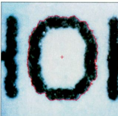
Photo 4: To measure edge roughness, we compare the perimeter of the original object to the perimeter of a smoothed version.
