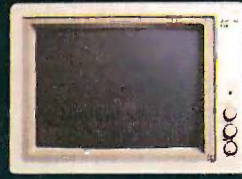
CM-1322 13" RGBI High Resolution 16 color display with 640 x 200 line resolution.
