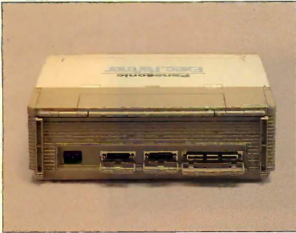
The back of the Exec. Partner showing, from left to right: power plug receptacle, parallel port, serial port, and expansion connector.
