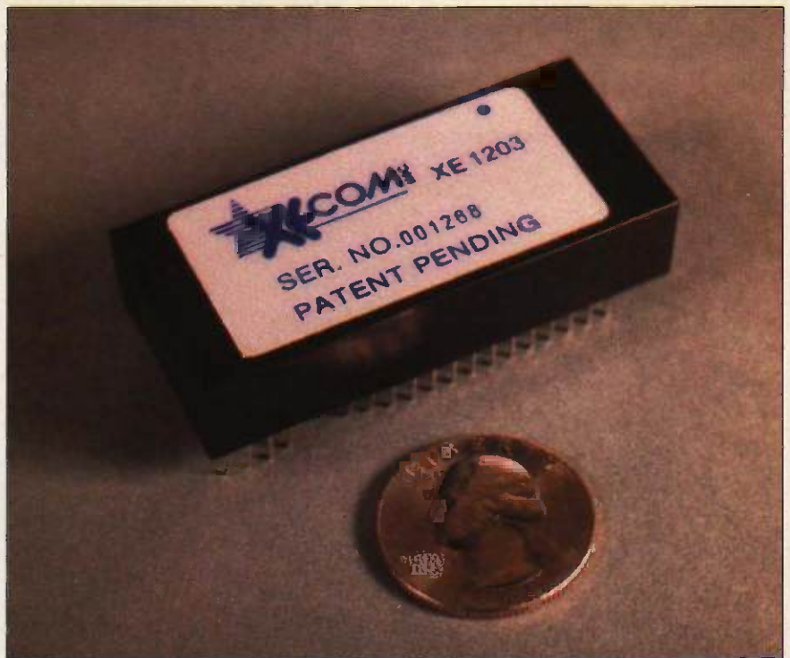
Photo 1: A close-up of the MOSART module as a 1200-bps modem (and more) on a chip.
