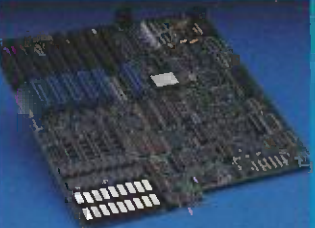
6 or 8 MHz 80286 motherboard, 640K standard memory, upgradable to 1M, clock calendar, fully compatible.
