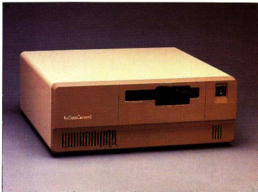
Photo 3: The Data General/One's optional expansion chassis, which includes a 5¼-inch floppy-disk drive.
