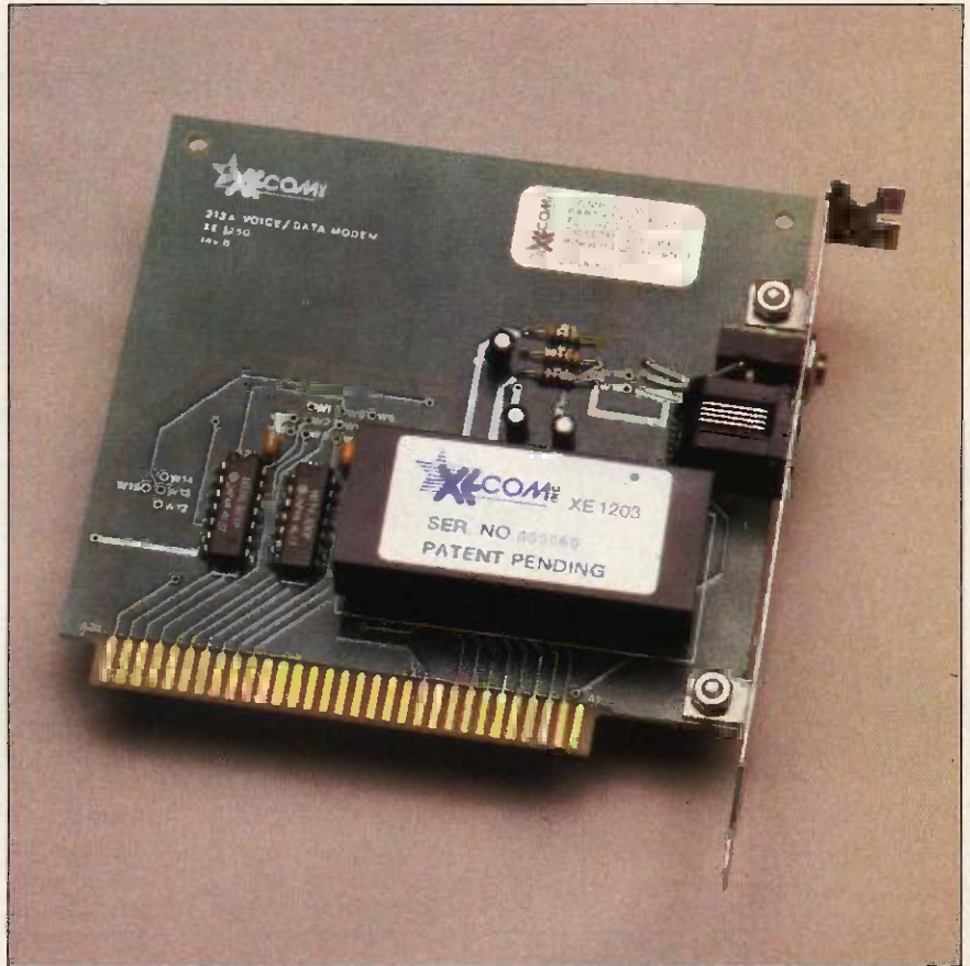
Photo 2: The Xecom IBM PC MOSART evaluation board.
