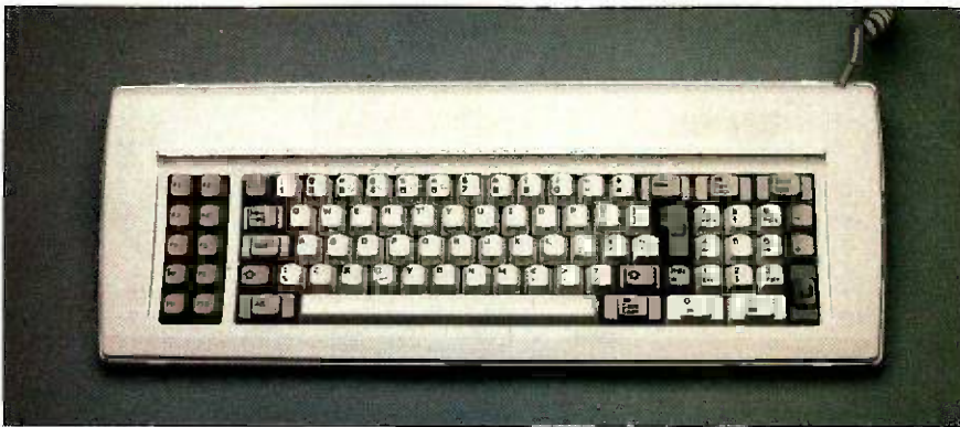
Photo 2: The keyboard of the Sanyo MBC-775. Note the LEDs in the Caps Lock and Num Lock keys and the second return key below and to the right of the numeric keypad.
