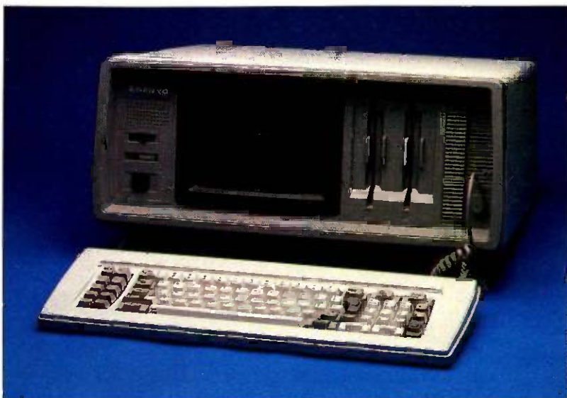
Photo 1: The Sanyo MBC-775 with built-in color monitor, keyboard, and two floppy-disk drives.
