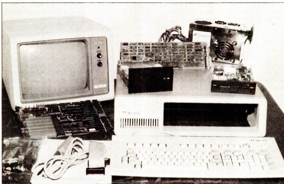
The FD-1000 kit for building an IBM PC XT-compatible computer.
