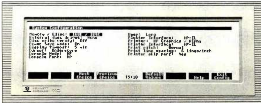
Photo 4: The system configuration menu. Using the function keys, it's possible to toggle among a full range of choices for each topic.
