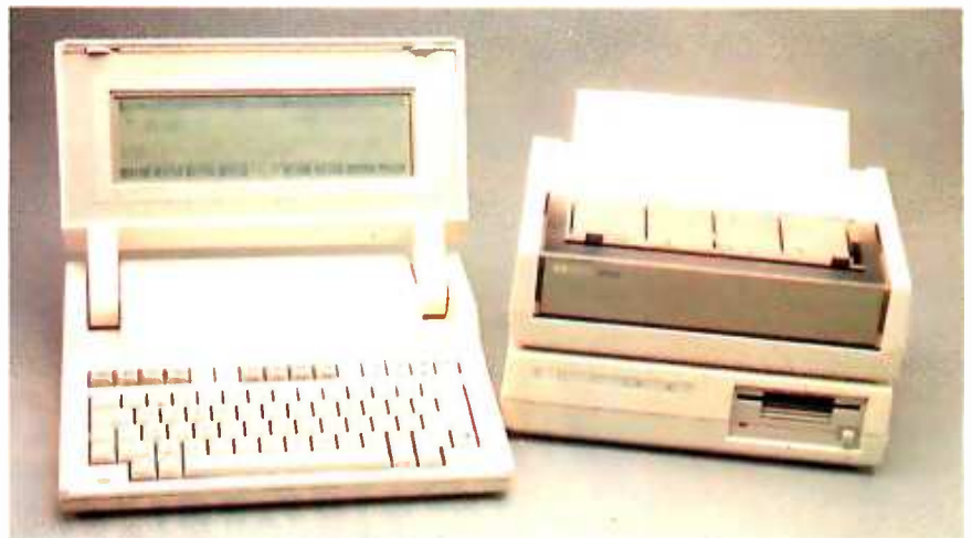
Photo 1: The HP 110 links to two optional battery-powered peripherals, the HP 2225B ink-jet dot-matrix printer and the HP 9114 single 3½-inch disk drive.
