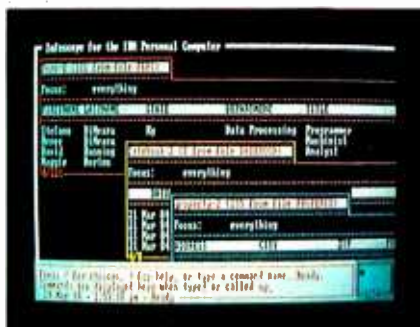
Photo 1: Scopes. Infoscope's name for windows, can be colored and then referenced by the color name rather than by the filename. On this screen, for example, the scope at top left could be moved to the cursor position with the command "move red here."
