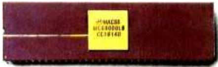
Macintosh's 32-bit MC68000 microprocessor.
