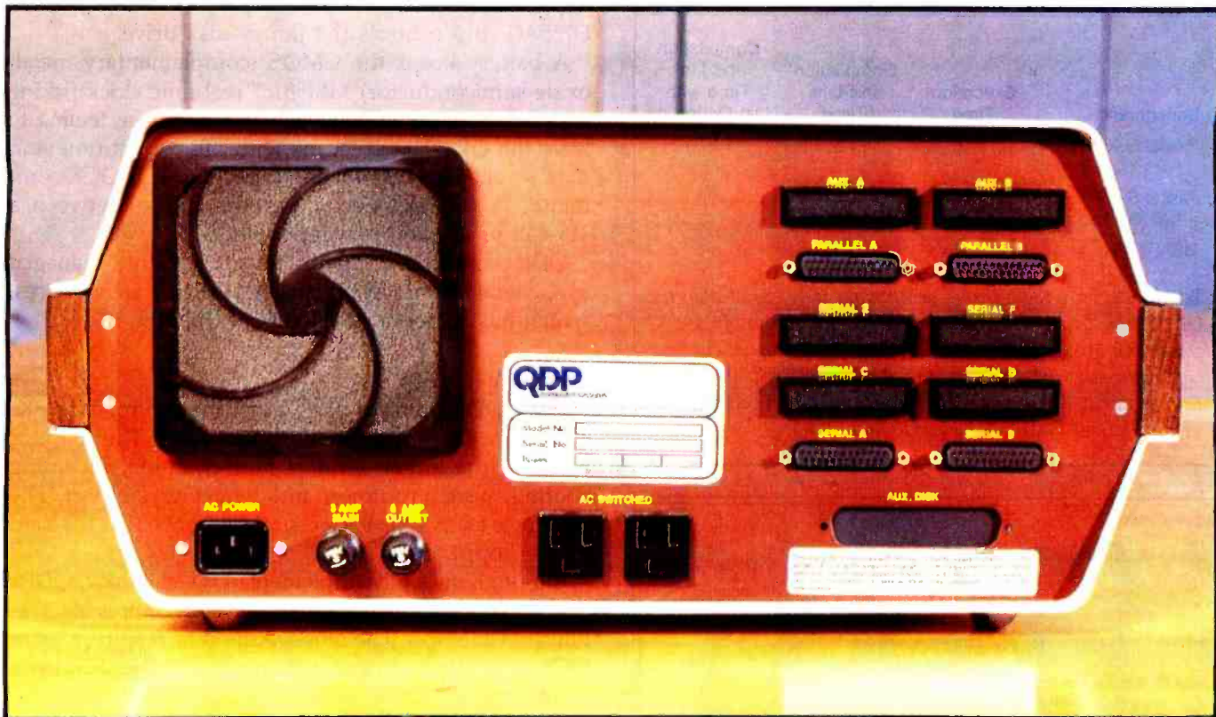
Photo 2: The back of the QDP-300. Two RS-232C serial ports and two Centronics-compatible parallel ports come standard with the system.
