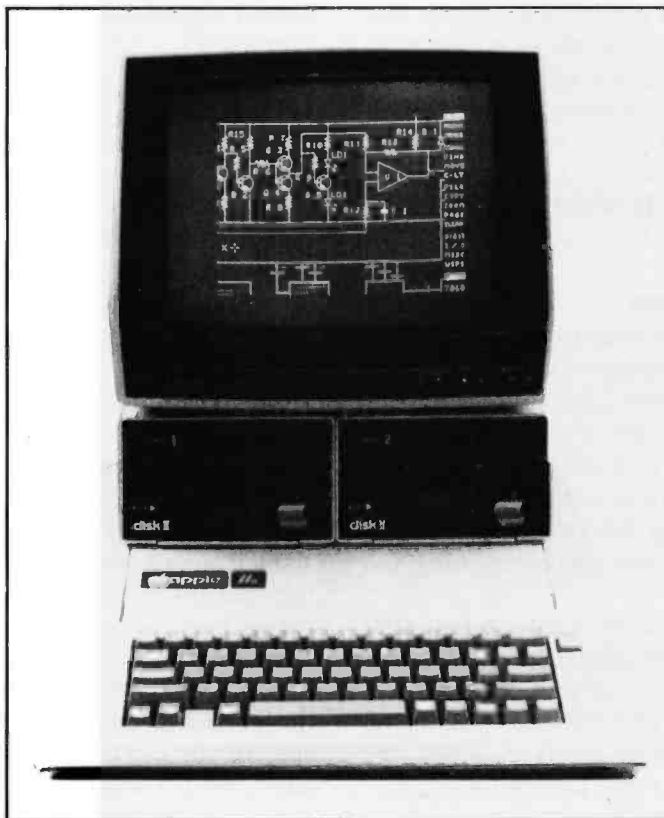
Photo 1: An Apple IIe displaying a typical CAD-1-created drawing.
