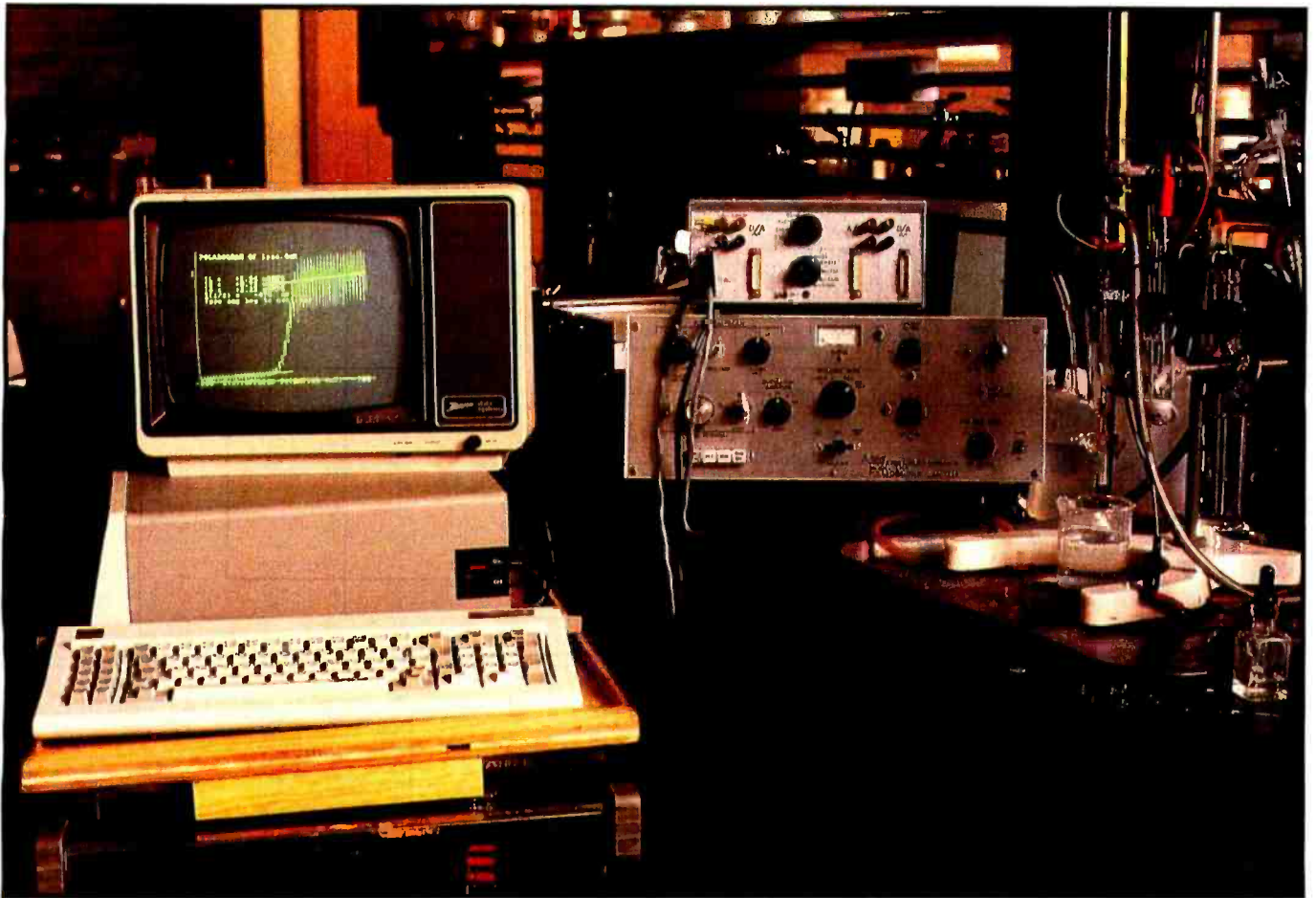
Photo 1: The general-purpose laboratory interface station can be moved easily from instrument to instrument because it is on a laboratory cart. The IBM PC contains a color/graphics monitor board and a Tecmar Lab Master interface board. The preamplifier box is perched on top of the larger control device for the polarograph, in the center. The electrodes for the polarograph are at the right side of the photo.
