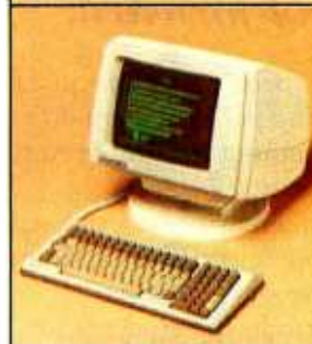
VIEWPOINT™/90. OEM's delight... double-high / double-wide, split screen, programmable function keys, down-line loadable, and more.
