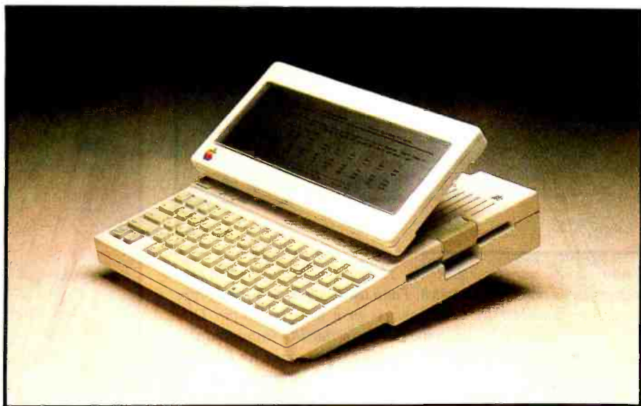
Photo 3: Apple has announced that a full-screen (560-by-192-pixel) flat-panel LCD will be available for the IIC before the end of 1984. The flat-panel display will support all the IIC's text and graphics modes and draw its power from the video expansion port.
