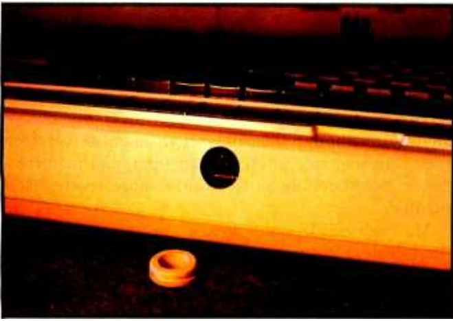
Photo 5: The APC nonmaskable interrupt switch. Access to the switch is possible only by removing a rubber plug in the rear of the keyboard.
