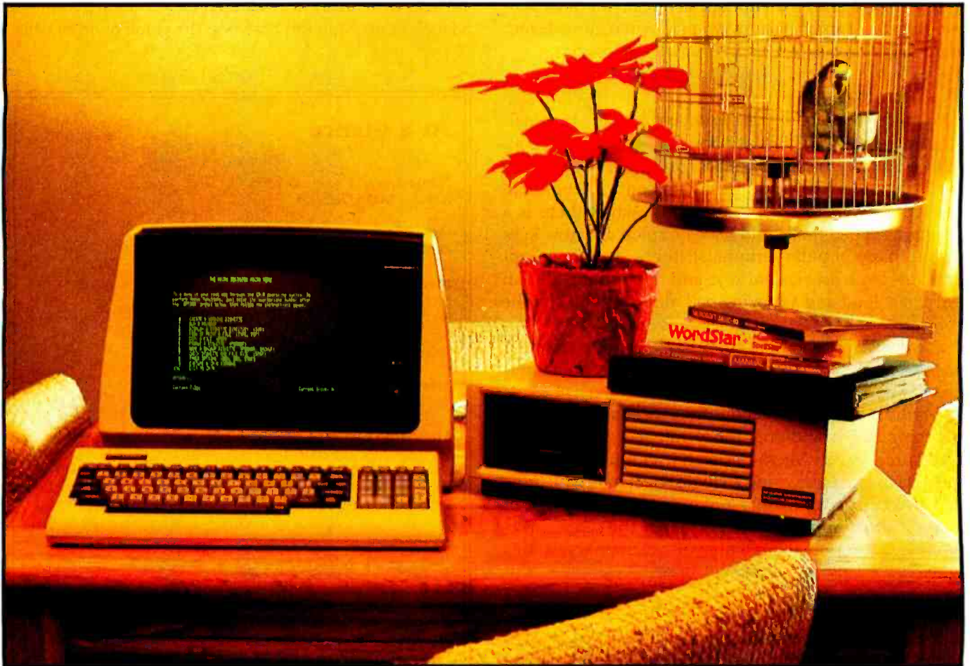
Photo 1: The Morrow Micro Decision. The system consists of a single-board computer based on Zilog's Z80 processor, some number of 5¼-inch floppy-disk drives, and a Lear Siegler ADM 20 terminal. At press time, Morrow planned to offer a Freedom terminal with the system instead of the Lear Siegler terminal.
