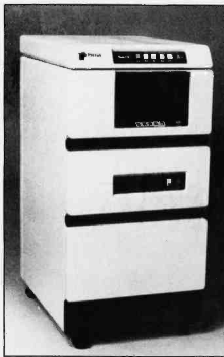
Photo 2: Plexus' P/40 uses multiple Z8000 microprocessors to achieve performance approaching that of a VAX.
