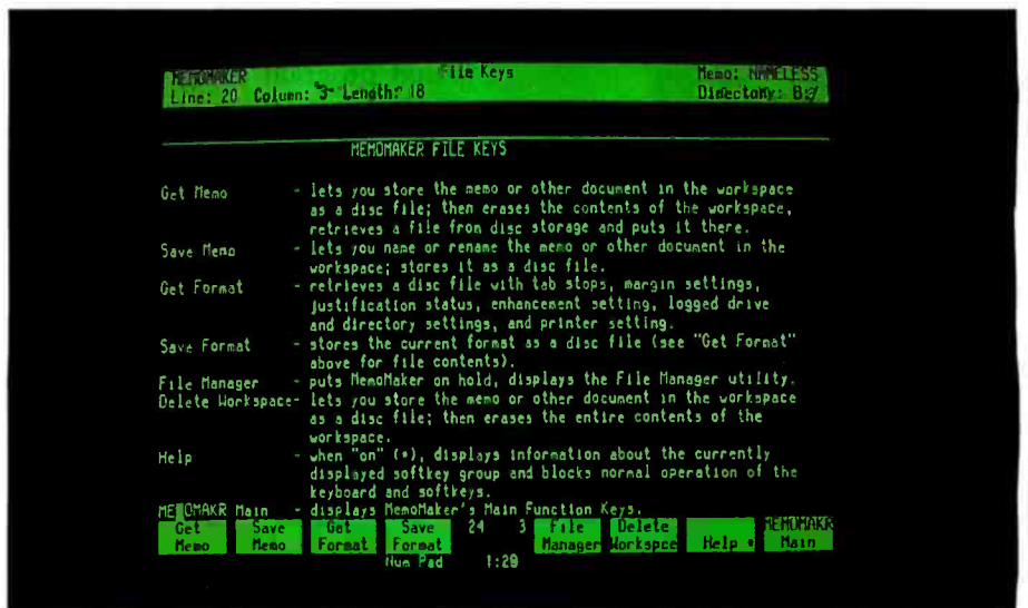
Photo 22: You can store memo formats in a separate file and read them into Memomaker. The asterisk in the Help softkey shows Help is toggled on.
