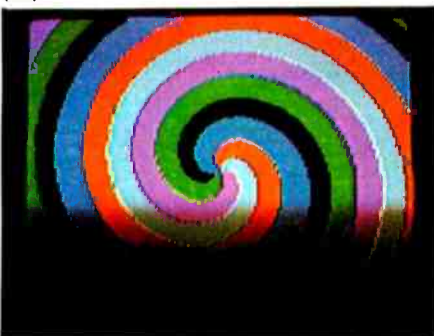
Photo 2: Video-display photographs illustrating the effects of camera timing. The 1/125-second exposure used to take photo 2a was too brief to record a whole frame. The shutter opened while the middle of the screen was being scanned and closed before the electron beam returned to the top of the screen. Note that the phosphor near the top was still glowing during the exposure even though the electron beam had passed on. In taking photo 2b, the timing control was set between 1/60 and 1/30 second; thus, some screen areas were scanned twice while the shutter was open, some only once. To take photo 2c, the camera was set for a 1/30-second exposure. Every part of the screen should have been scanned exactly twice while the shutter was open. Unfortunately, the camera's timing mechanism is not sufficiently precise for this purpose.
