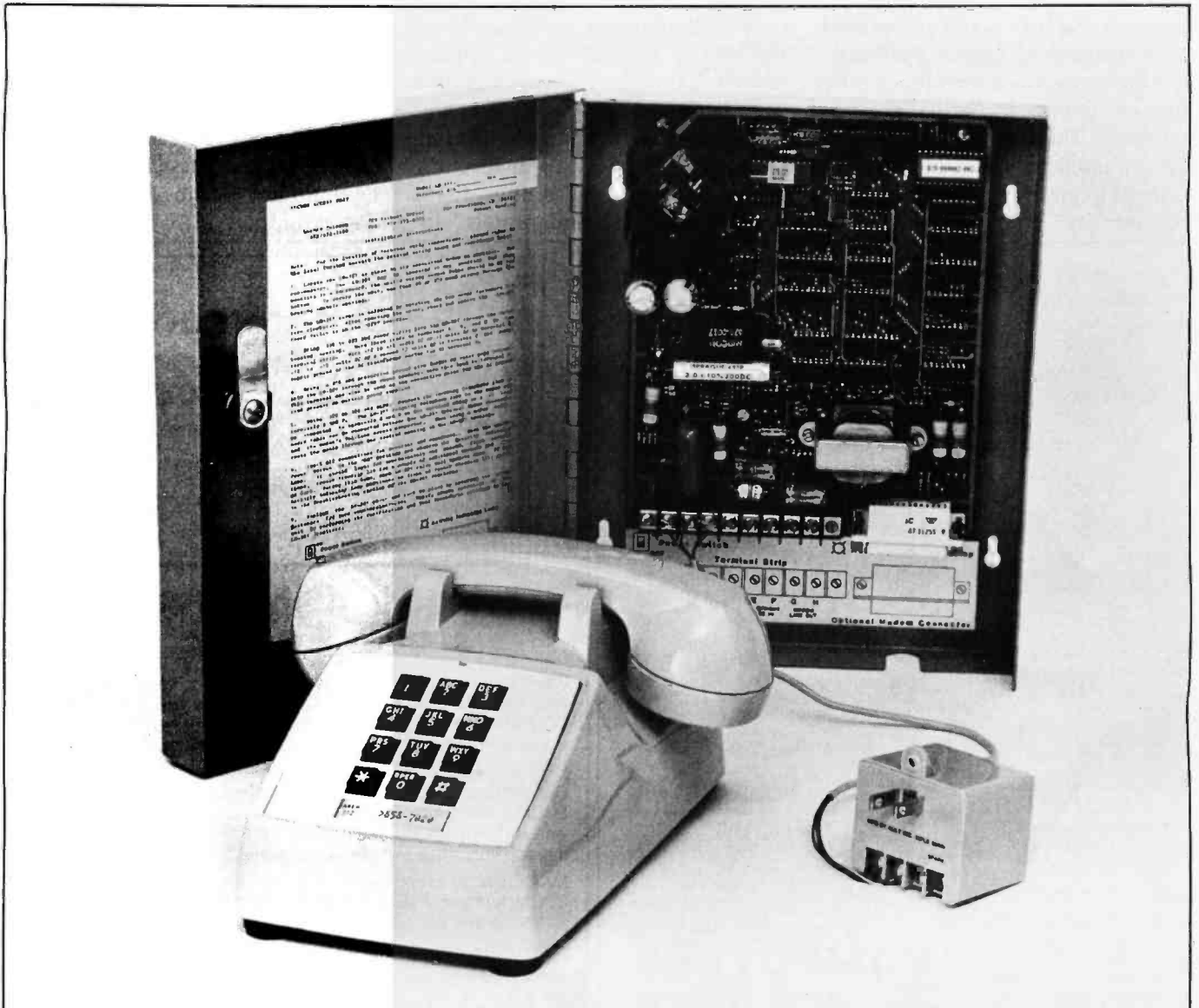
Photo 1: The Secure Access Unit works with a telephone and modem that provide direct-dial access to a computer. It calls back a remote terminal to verify that the user is requesting access at an authorized location.
