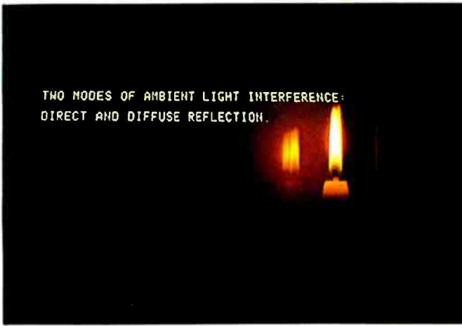
Photo 3: Video display with candle, resulting in two sharp reflections of the candle's flame: one from the front surface of the glass screen and another from the back surface. Light from the flame also scatters back from the phosphor in all directions.
