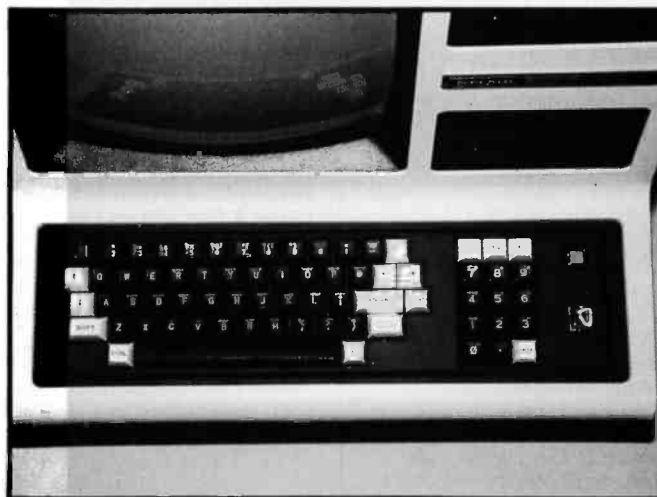
Photo 3: The Model 4's keyboard enhances the Model III's with a caps lock, control key, and three function keys.
