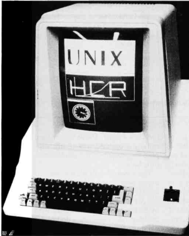
Photo 1: The NS16000 workstation, which includes memory-management and floating-point capabilities. This workstation was used to port a demand-paging virtual-memory implementation of Unix to the NS16032 processor.
