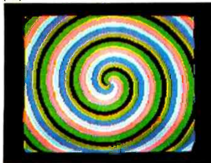
Photo 2: Video-display photographs illustrating the effects of camera timing. The 1/125-second exposure used to take photo 2a was too brief to record a whole frame. The shutter opened while the middle of the screen was being scanned and closed before the electron beam returned to the top of the screen. Note that the phosphor near the top was still glowing during the exposure even though the electron beam had passed on. In taking photo 2b, the timing control was set between 1/60 and 1/30 second; thus, some screen areas were scanned twice while the shutter was open, some only once. To take photo 2c, the camera was set for a 1/30-second exposure. Every part of the screen should have been scanned exactly twice while the shutter was open. Unfortunately, the camera's timing mechanism is not sufficiently precise for this purpose.
