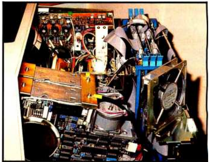
Photo 6: Inside the APC (color model). At left are the two 8-inch disk drives. To the right is the ventilation fan. Behind the fan is the six-slot card cage, presently occupied by three boards. To the left of the card cage is the CRT, and behind that is the main analog board.
