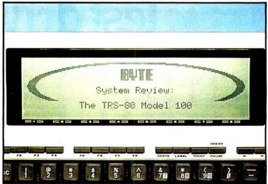
Photo 2: A close-up of the liquid-crystal display of the Model 100. The display size is 8 lines by 40 characters (64 by 240 pixels).
