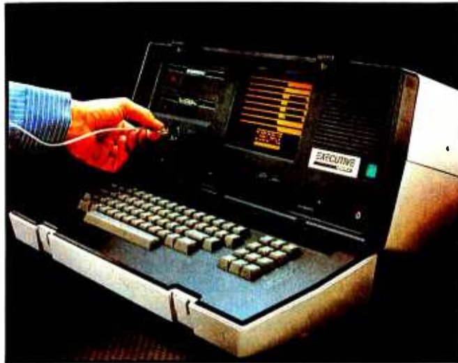
Photo 1: The Osborne Executive with a 7-inch amber screen, two half-height disk drives, and the input/output connectors across the bottom front of the computer.
