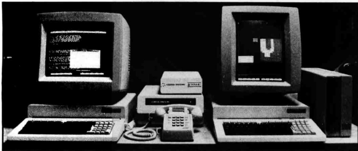
Photo 1: Two Concepts linked to a 6-megabyte hard-disk drive (center) via an Omninet local-area network. An 8-inch thin-line floppy-disk drive (right) is connected to a controller board installed in the Apple II-compatible expansion bus of the Concept on the right. The video display on the right is set up in the portrait format, almost the exact size and shape of a sheet of paper. The monitor on the left has been rotated 90 degrees for viewing in the landscape format.
