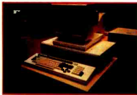
Photo 1: The Fortune 32:16 microcomputer with Motorola 68000 processor.
