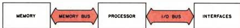
Figure 2: A computer system with an I/O bus in addition to a memory bus. Building in a separate I/O bus frees all the memory-address space for the processor's own use.
