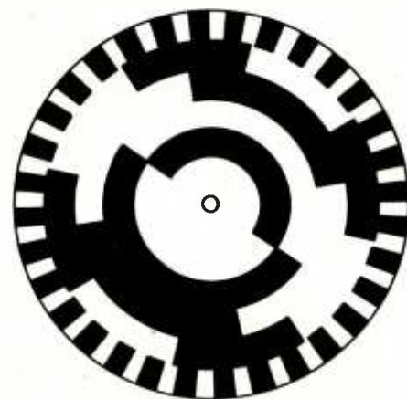
Figure 3: The optical encoding disc uses a Gray code to eliminate ambiguity in angular position of the wind vane, while in the anemometer only the outermost ring is used as a sort of tachometer.
