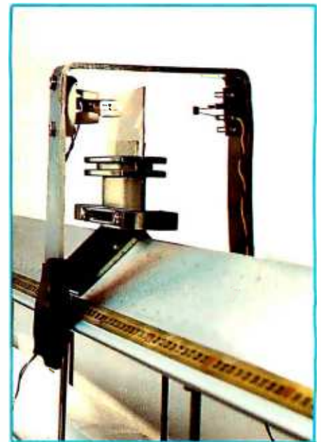
Photo 2: Lamp and phototransistor attached to one end of the air track. For best timing resolution, the lamp is mounted so that its filament is vertical.
