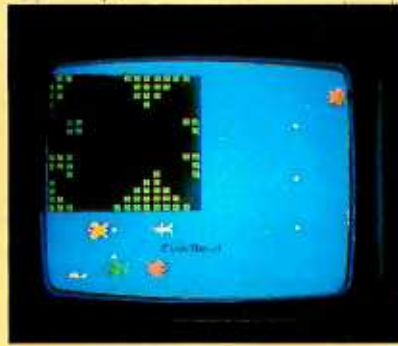
Photo 5: The shapes and characters used in the FISHBOWL (photo 5a) were specifically defined (see listing 1 for the procedures). Shapes are defined by blacking out the desired shape on a 16 by 16 square grid (photo 5b). Characters are similarly defined on an 8 by 8 grid (photo 5c).
