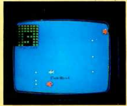
Photo 5: The shapes and characters used in the FISHBOWL (photo 5a) were specifically defined (see listing 1 for the procedures). Shapes are defined by blacking out the desired shape on a 16 by 16 square grid (photo 5b). Characters are similarly defined on an 8 by 8 grid (photo 5c).
