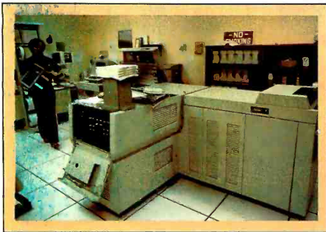
Photo 5: The Xerox 9700 high-speed printer used by Dialog for off-line printing of references. The printer operates at two pages a second and offers Dialog users a considerable savings over having their references printed out while logged onto the system. The average cost of having references printed off-line and mailed to you is $0.10 to $0.25 per citation.
