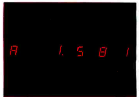
Photo 5: A measured time is read by pressing a letter key on the trainer's hexadecimal keyboard. This is the display's appearance when the A key is pressed to read out the elapsed-time measurement (here 1.581 seconds) stored at memory location A.
