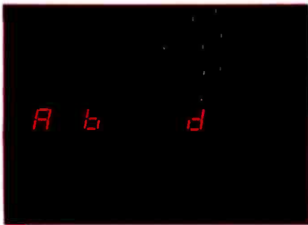
Photo 3: The trainer's six-character LED display is used to indicate which memory locations have been loaded with elapsed-time measurements. This is how the display appears after time measurements have been logged in memory locations A and B (for phototransistor 1) and location D (for phototransistor 2).
