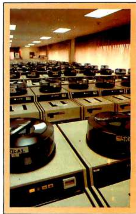
Photo 2: Some of the 200 hard-disk drives used by the Dialog system. Most of the CDC (Control Data Corporation) drives hold 637 megabytes of data for a total of more than 50 billion bytes of on-line storage.
