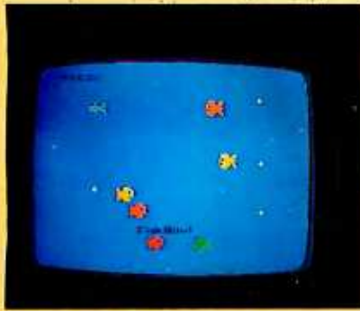
Photo 5: The shapes and characters used in the FISHBOWL (photo 5a) were specifically defined (see listing 1 for the procedures). Shapes are defined by blacking out the desired shape on a 16 by 16 square grid (photo 5b). Characters are similarly defined on an 8 by 8 grid (photo 5c).
