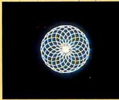
Photo 10: The SPINSLINK figure (photo 10a) is the result of the simple five-line SPINSLINK procedure (shown in the edit mode in photo 10b) that calls the three-line RCIRCLE procedure which, in turn, calls the RCP procedure. Each procedure is nested in the one listed below it. Note the use of floating-point arithmetic in RCP, the use of iteration in RCIRCLE, and the use of recursion in SPINSLINK (it calls itself). (The procedures are taken from the draft of the Apple Logo manual prepared by Harold Abelson.)
