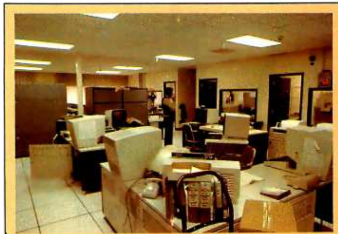
Photo 1: The Lockheed Dialog computer room operator station. The system uses two mainframe computers—an IBM 3033 and an AS-9000 (sold in the United States by National Advanced Systems). Each computer contains a complete Dialog operating system; one handles Telenet calls, and the other Tymnet. Direct dial-in calls and leased lines are divided between the computers to even the loads. Because of the large amount of computer power available, the average wait for a response to a query is ten seconds—despite the fact that hundreds of users may be logged in during peak-use periods.
