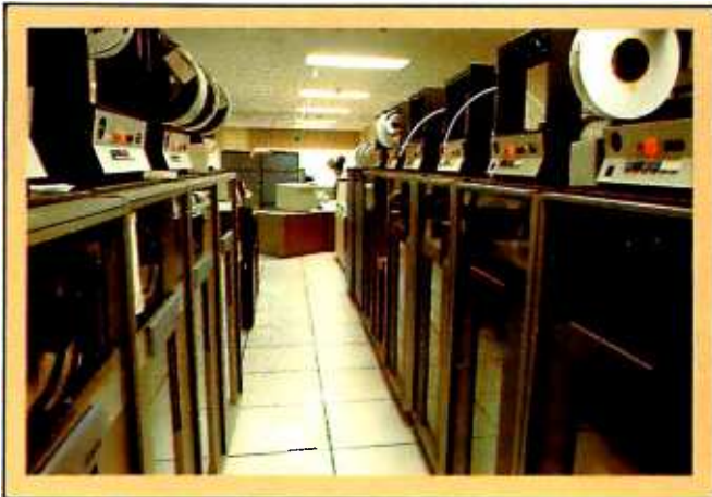
Photo 4: IBM reel-to-reel tape drives used to load new and updated information into the Dialog disk drives.
