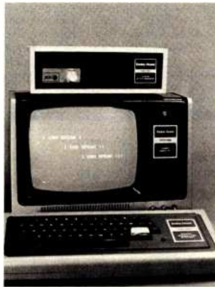
Photo 1: Radio Shack TRS-80 computer system with the voice synthesizer module sitting on top of the video monitor.
