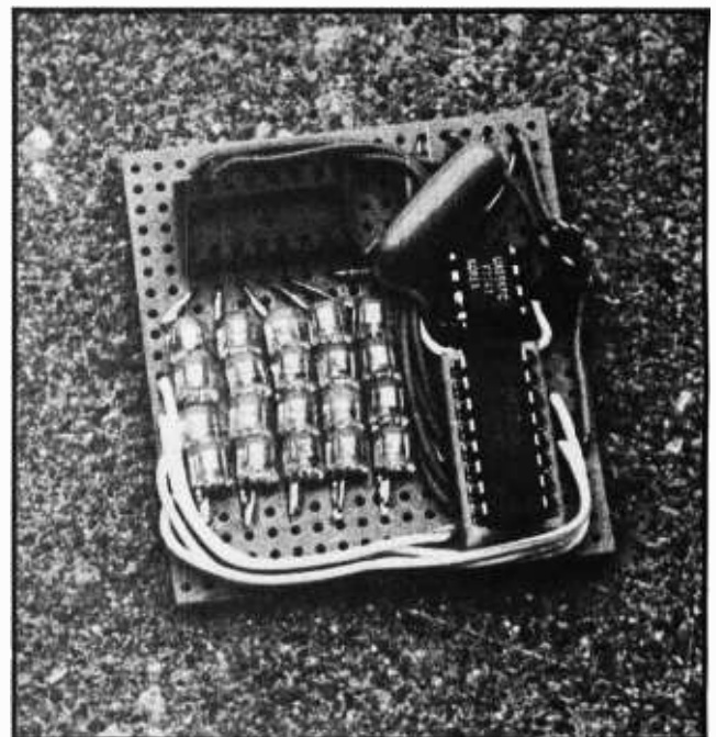
Photo 4: Interior of the sustained contrast detector. Shown at (a) is the lens (at left), the array of phototransistors (at right), and the associated electronics. 4b shows the 4 by 5 prototype array (compare with final version in figure 7).
