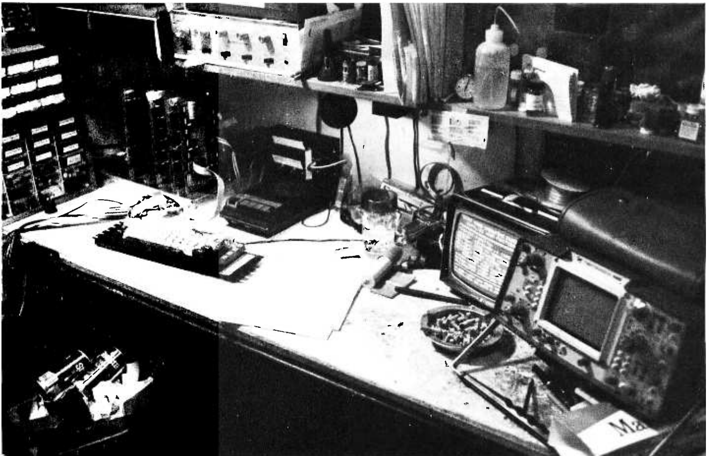
Photo 21: A Microcomputer Development Workshop? The processor is off in the left hand corner of the table, with a cassette tape recorder to its right. A keyboard with ASCII encoding is connected to the IO card for control of the processor. The video display's television set output is to the left of the oscilloscope at the right side of the picture. The parts cabinets, wire wrap gun, soda pop and ash tray were essential to the development of this system.
