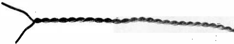
Photo 3: Twisted pair cable is the only good data transmission line which can be easily fabricated at home. Here is an example made using an electric drill to do the twisting.
