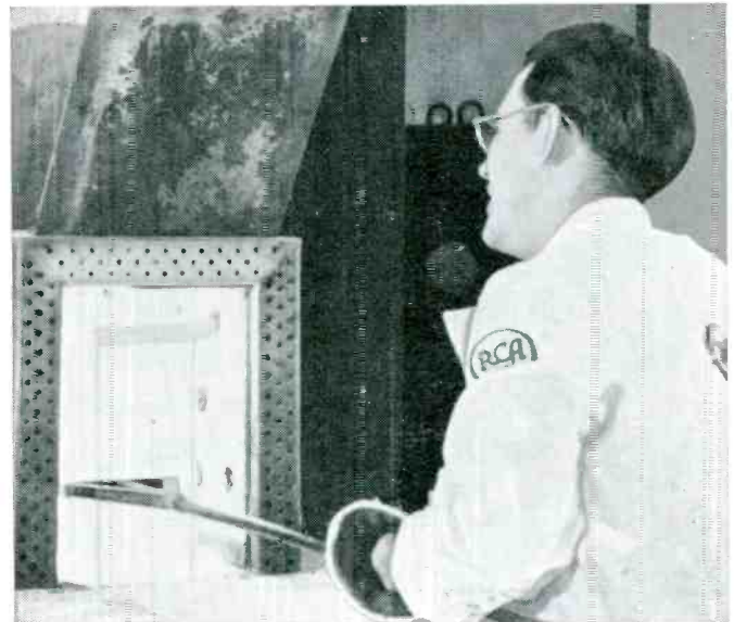
After this white-hot block of luminescent material is taken from the furnace, it will be spread on the face of a kinescope to form the screen for television pictures.
