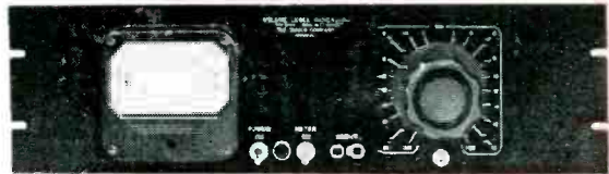
Type 920 Rack model, low-level bridging type. Meter multiplier range: —20 VU to +20 VU. Power supply, 100—130 V, 60 cycle AC, with voltage regulator for normal variations. Reference level: 1 mv into 600 ohms. Special ranges on request.
