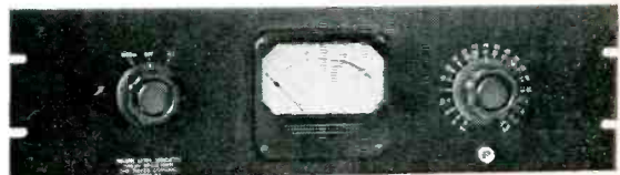
Type 915 Rack model, terminating and bridging type. Meter multiplier ranges: Terminating, —6 VU to +32 VU; bridging +4 VU to +2 VU; or terminating, —6 VU to +16 VU; bridging, +4 VU to +2 VU. 2 VU steps. Reference level: 1 mv into 600 ohms.
