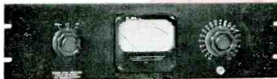
Type 915 Rack model, terminating and bridging type. Meter multiplier ranges: Terminating, —4 VU to +22 VU; bridging —4 VU to +42 VU; or terminating, —0 VU to +16 VU; bridging, +4 VU to +26 VU. 2 VU steps. Reference level: 1 mv into 600 ohms.
