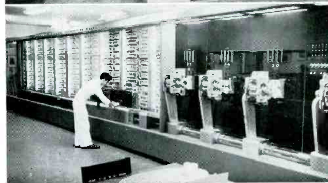
(Bottom)—I.B.M. Automatic Sequence Controlled Calculator. Fifty foot long electrical computer at Harvard University.—(Credit Harvard News Service.)
