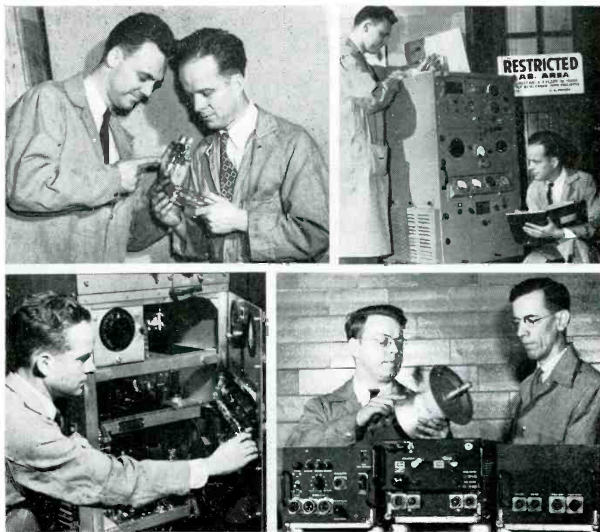
Top left (Fig. 4): The CW magnetron, designed and developed by General Electric, is the heart of the radar jammers used by the Navy and the Air Force. Engineer L. M. Ewing (l.) points to a production line magnetron. Engineer J. W. Downie (r.) holds the original CW magnetron which was designed by G-E according to Navy specifications in one Saturday afternoon in 1944. Ten days later, mass-produced magnetrons were in radar jammers en route to the Pacific. Top right (Fig. 2): General Electric's radar jammer, the TDY-2. Engineer L. M. Ewing (l.) inserts G-E designed and developed CW magnetron in the jammer, while Engineer J. W. Downie makes a reading from the dials.
