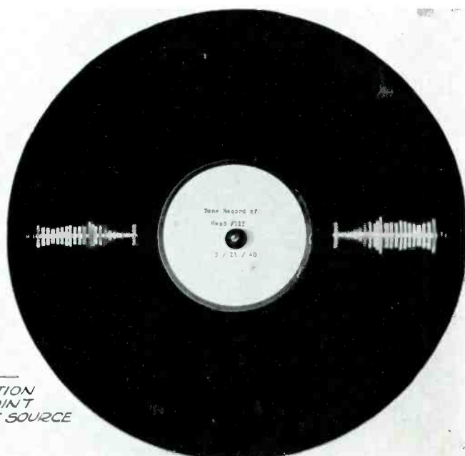
FIG. 8. Variation of optical patterns of typical tone record
