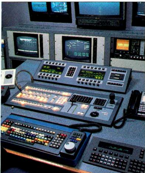
106 Abekas Video Systems A84 4:2:2 Digital Production Switcher.
