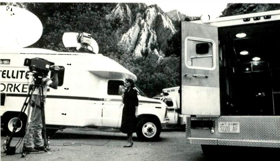
Centro's Satellite Networker is equipped with a 2.3-meter antenna that folds down into the vehicle's roof for an overall height of 11 feet.
