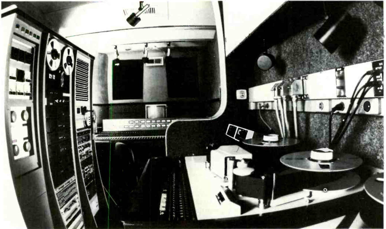
An MCI board and two Ampex 24-track recorders are part of the equipment on board Westwood One's Concertmaster truck.
