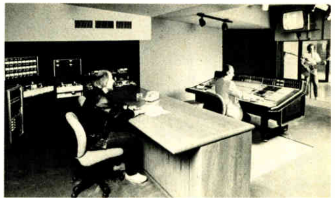
A complete audio recording studio allows full sweetening functions with an SSL 6000E console, Eclipse synchronizer, and Studer multitrack recorders.
