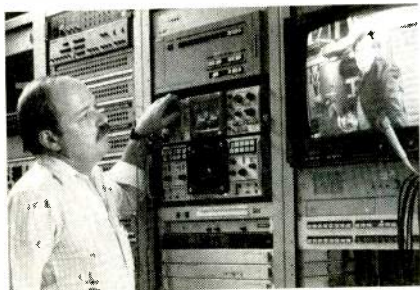
A Sony BVX-30 digital noise reducer cleans up WNOL's signal before transmission.
