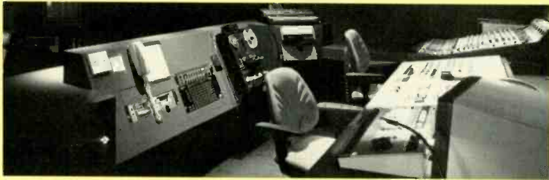
VideoWorks' Edit Room One features a CDL-480-8 switcher, ADO and NEC digital effects, and a Yamaha mixing console.
