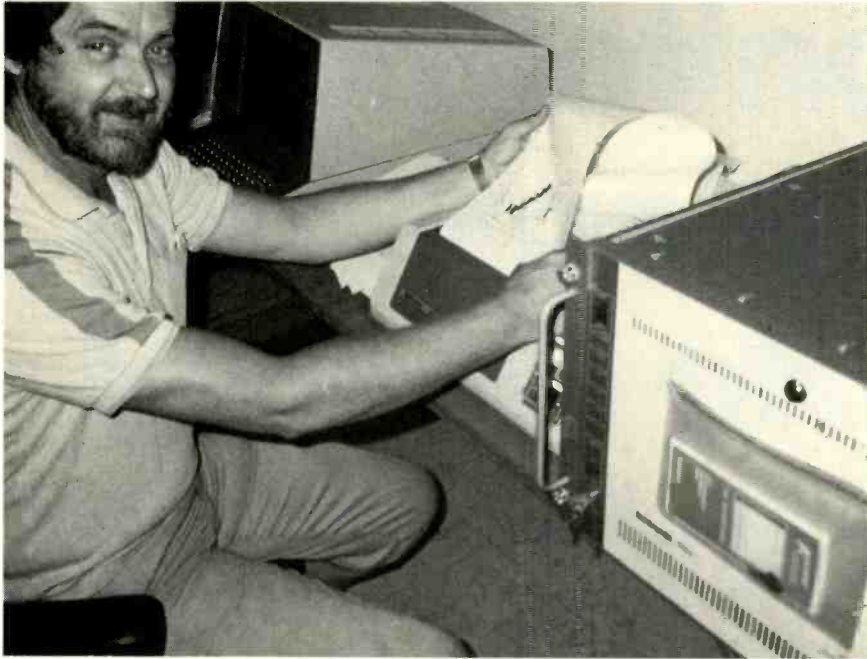
An operational ANSWER system at the Atlanta transmitter site near Lexington, NE. Shown from left to right are the Tektronix 4006 Computer Display Terminal, 4631 Hard Copy Unit, and the ANSWER Unit.
