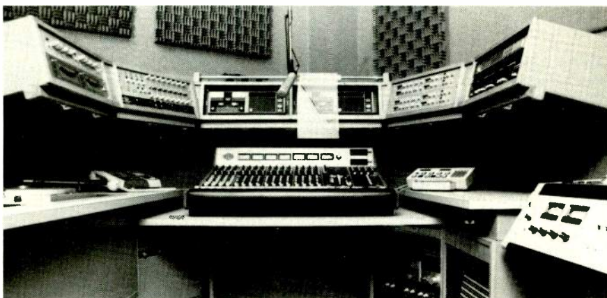
Q-94's new semicircular production room, with a Quad/Eight 248 console and Otari recorders.
