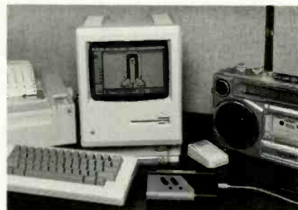
The only special equipment necessary for radio listeners to download Microperipheral's programs and graphics is a 4800 baud modem.
