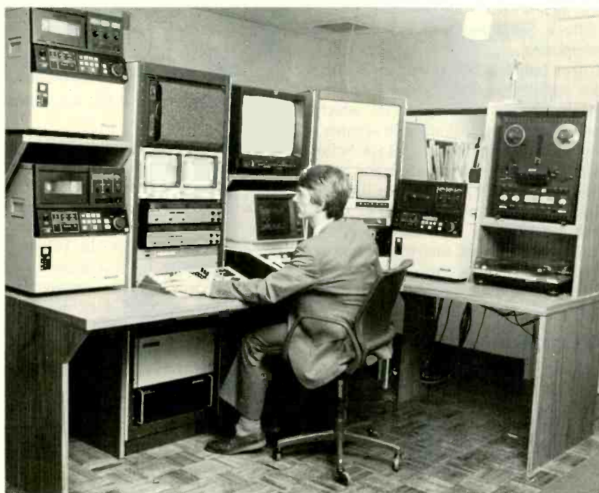
Karl Renwanz, WNEV's VP of engineering and operations, in one of the station's five component editing suites which feature M-format decks, Fortel TBCs, and R,G,B monitoring.
