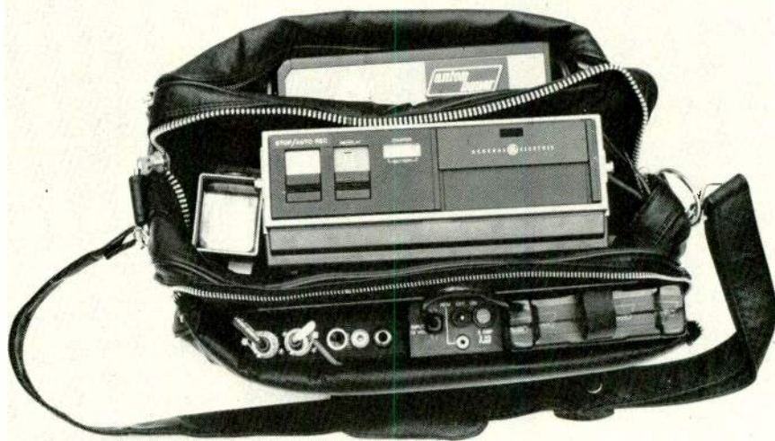
Anton/Bauer's Spy Cam system, designed for covert newsgathering, is a leather unisex shoulder bag containing (top to bottom) camera with Newvicon pickup tube and special pinhole lens; compact VHS recorder with special "auto record" mode and mini-monitor with 1.5-inch display; and Anton/Bauer battery and charger.
