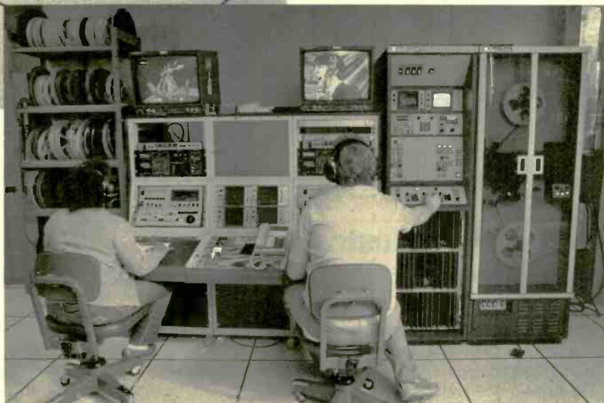
WNOL-TV transfers film to half-inch Betacam with its Rank Cintel, keeping the video in components.
