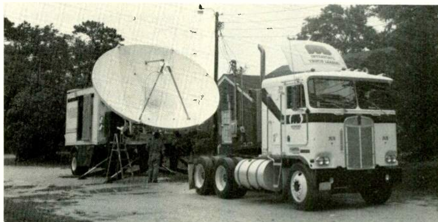
In Myrtle Beach, CBS's Ku-band uplink, courtesy of VideoStar, waits the last few hours for hurricane Diana.
