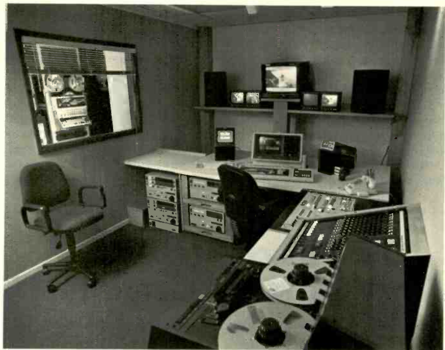
Rock Solid Productions' on-line edit suite features a Grass Valley 1600 1X switcher, a Chyron CG with R,G,B output, an ISC edit controller, R,G,B monitoring, and Betacam recorders.
