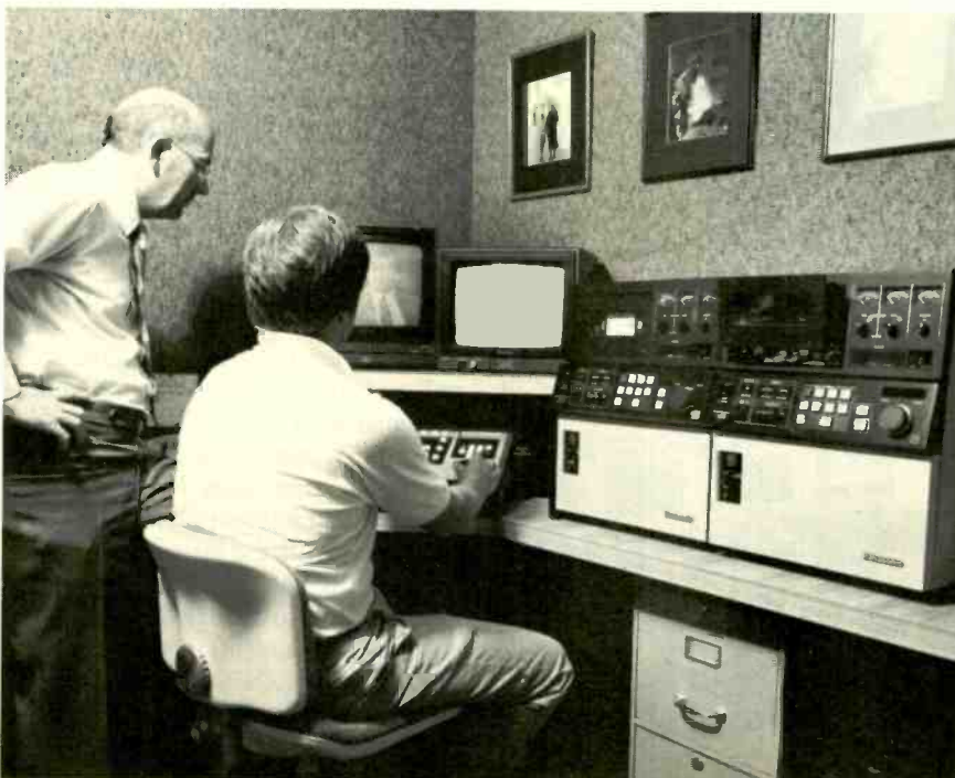
At WGRZ-TV, Buffalo, NY, cameramen edit their own footage on M-format machines. The station has six component edit rooms, with Fortel component TBCs.
