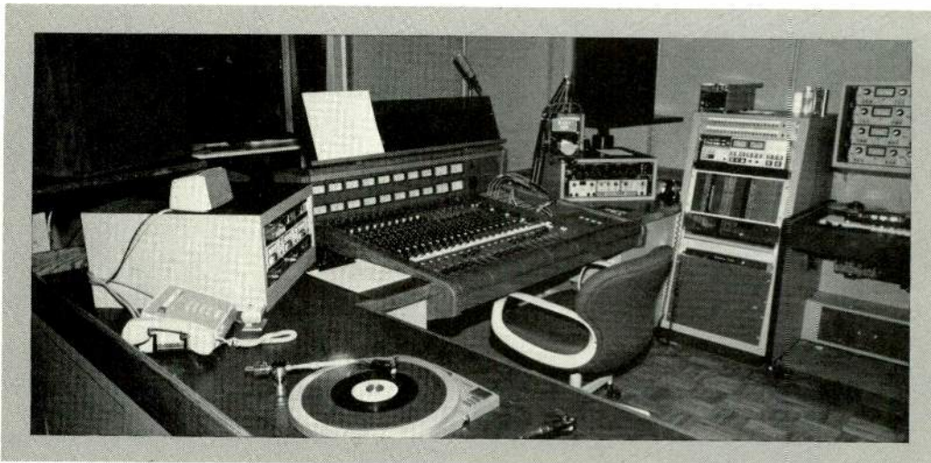
WAXY's state-of-the-art studio, built around MCI 618 audio board, features multitrack recorders.
