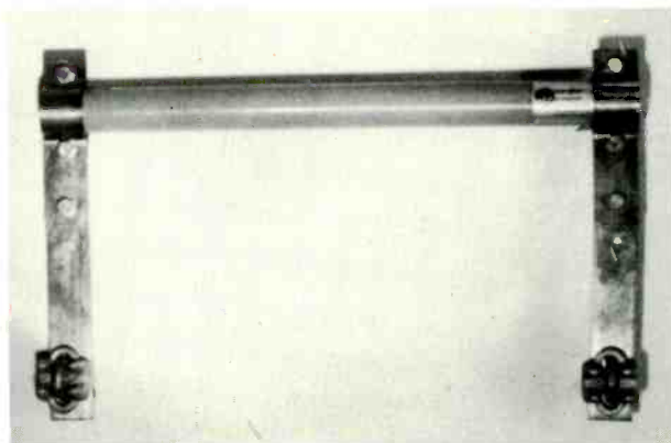
Dissipation choke from LEA carries lightning-induced energy around guy wire insulators, but has high impedance to the RF energy.
