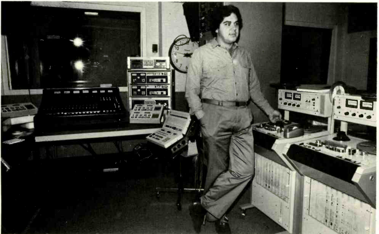
The travelling studio at ABC consists of a Yamaha console, ITC carts, an Otari auto-locator for MTR-10s, and a rack including Lexicon digital processors.
