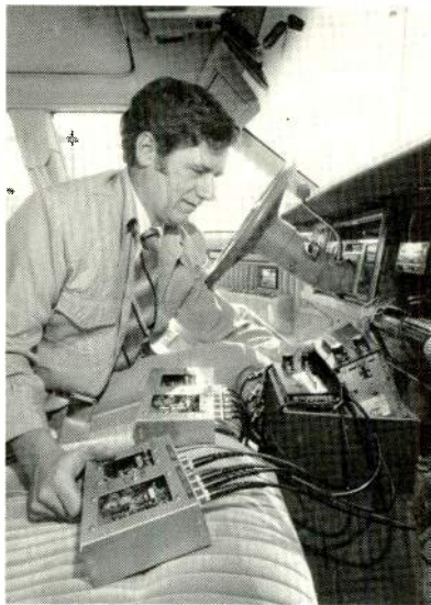
Engineer Keith Schultz installs Delco-GM receivers and AM stereo decoders (on seat) in 1982 Cadillac Seville for AM stereo field tests.
