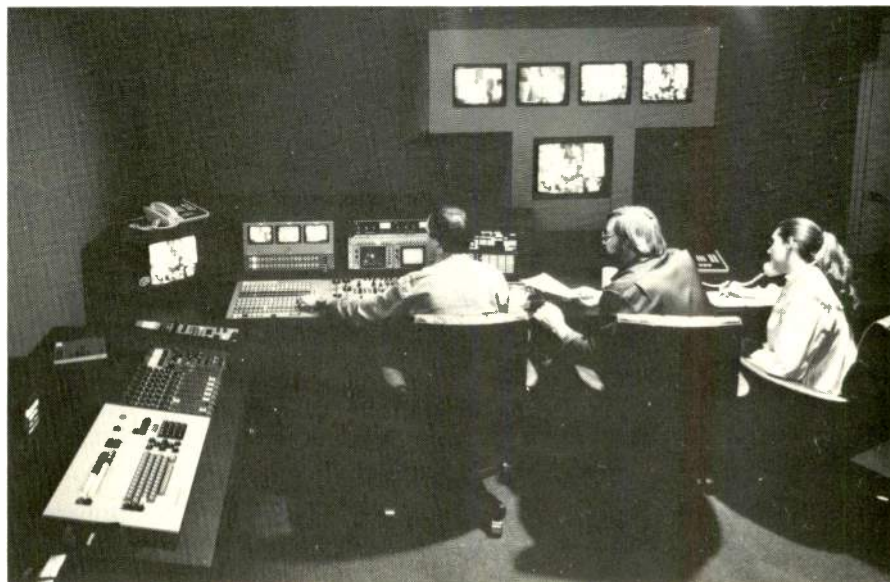
At Scene Three's current facility, one-inch video edit suit features a CMX 340X editing system and two-channel Vital SqueeZoom.
