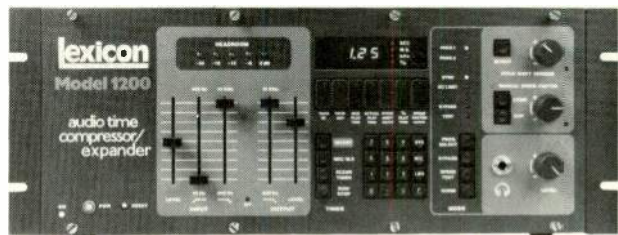
The audio time compressor/expander from Lexicon is a dedicated computer with keypad control of all playback parameters.
