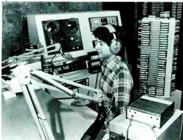
Main control uses stand-up operation, with cart machines flanking console at each end, reel-to-reel machine at right, carts for music and spots in back of operator.
