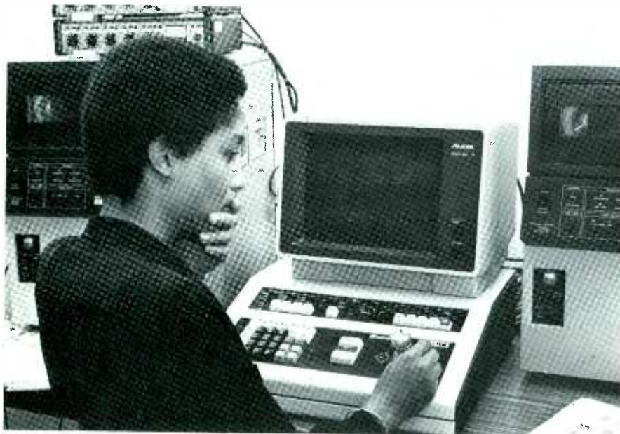
In another Look edit room, operator edits a segment on Convergence ECS-103B. Amdak monitor displays edit menu.
