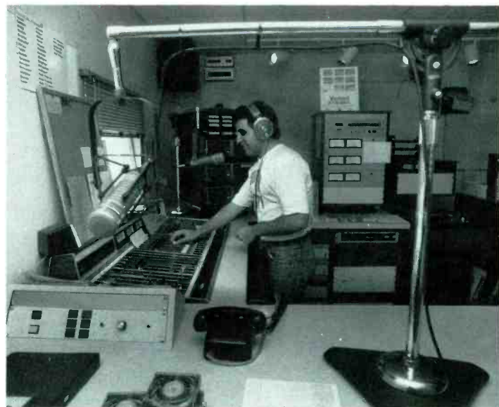
FM jock John Dowd with Belar modulation monitors and Moseley remote units, seen to his right. The E-V RE20 microphones are used throughout the station.
