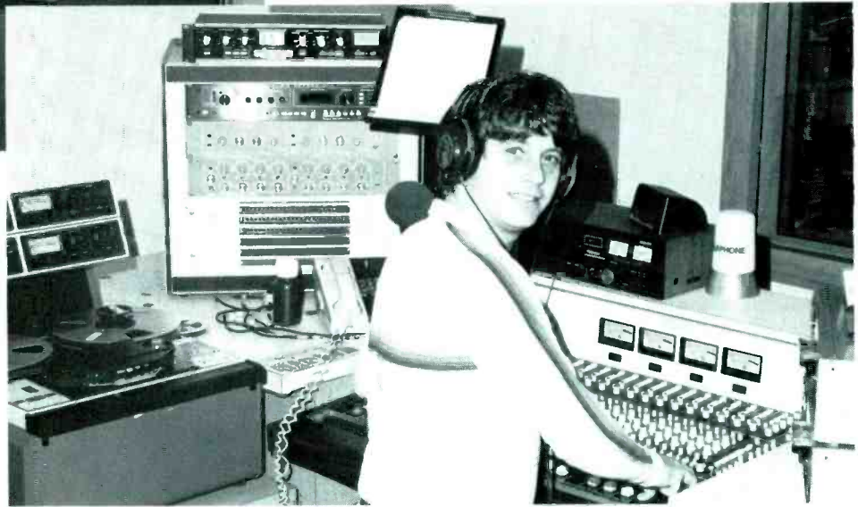
In WJYN's production studio, an Ampex ATR-100 half-inch, four-track deck and an 18-channel Audiotronics console give operator Doug Remington complete freedom during mixdown.
