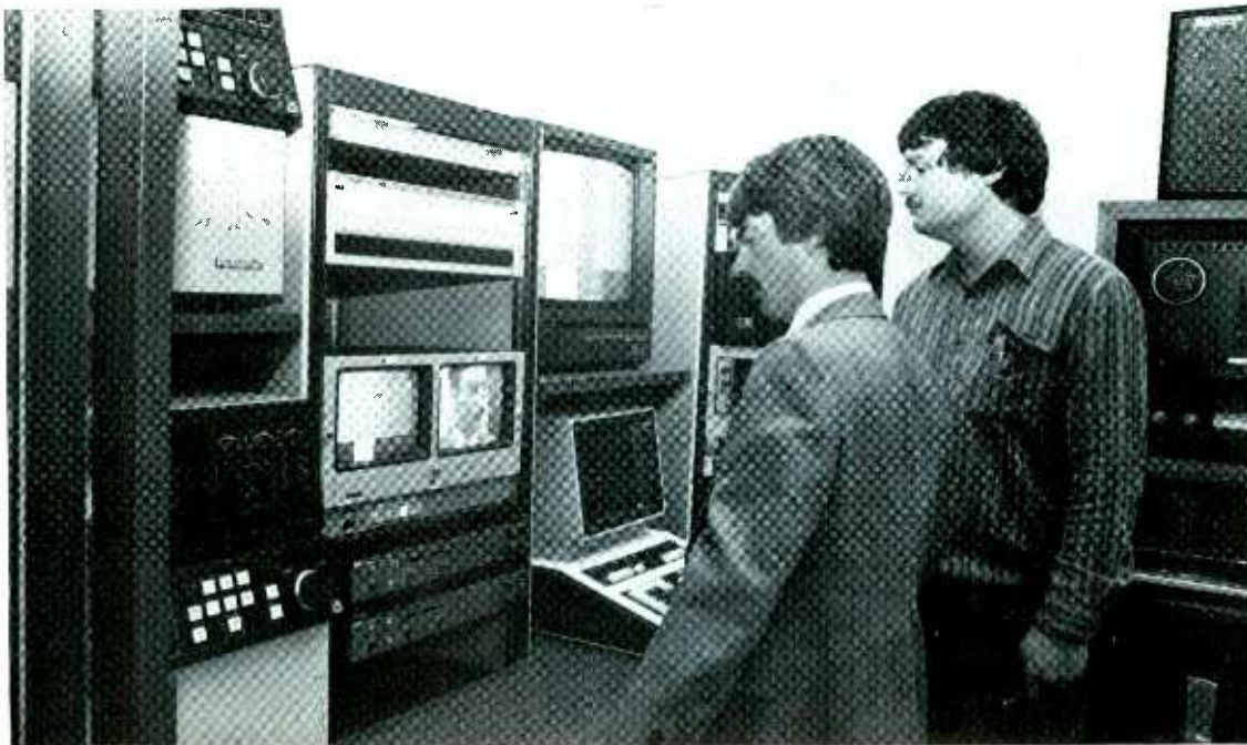
Chief engineer Renwanz (left) and engineering manager Lay check the signal in the main edit room for Look . Fortel TBCs are just below twin monitors.
