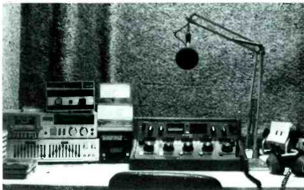
Newsroom isolation booth employing the LPB console and ITC cart deck.
