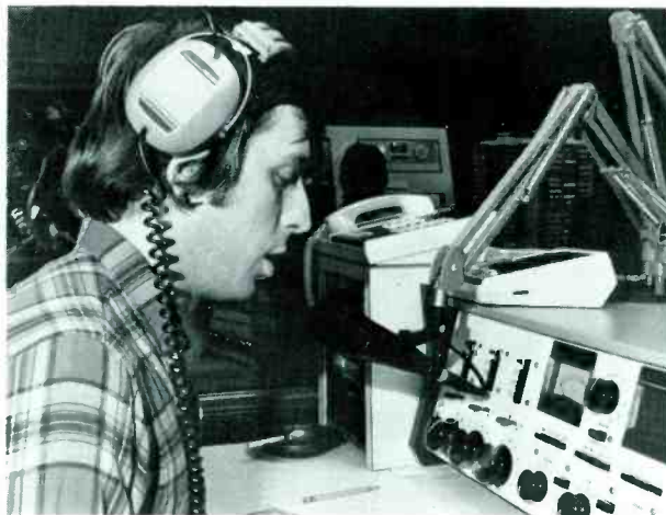
Newsman goes on the air from the news booth, built around an Ampro console, using Sennheiser mic. Boom for one of additional mics, for conference guests, is at extreme right.
