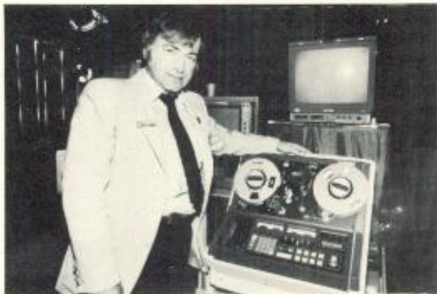
Bob Cezar shows the IVC-1, which records R, G, and B components separately.
