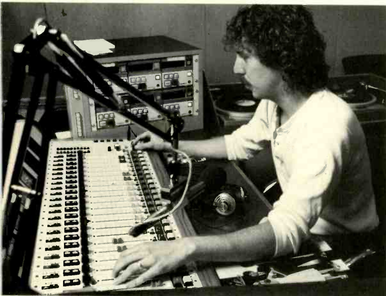
In one of RKO's control-room-studios, Barry Luchkowec operates Pacific Recorders' BMX console. Six Tomcats, Pacific Recorders' cart machines, are at his right
