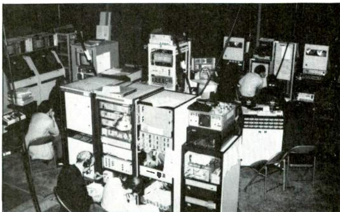
The digital component encoding demonstration. In the center of the room, the racks house the Dynair switcher, the VG zone plate generator, and various pieces of test equipment. To the left are the Ampex VTRs, in the back the Sony DVRs, and in the forefront the CCU for the RCA TK 47
