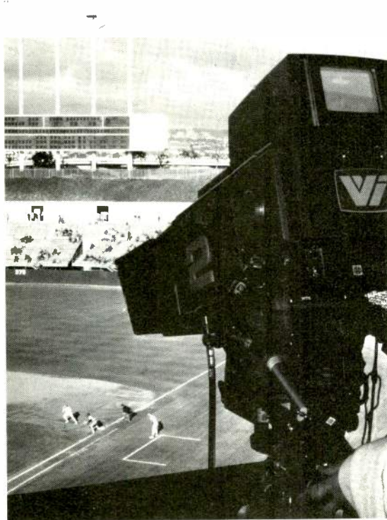
While the Sportsfocuser must be pointed down toward a flat playing field, it can be switched out of function quickly for other shots
