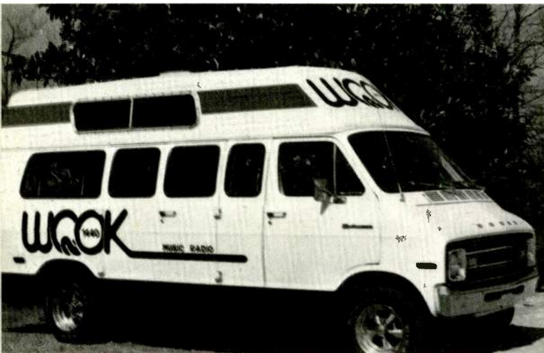
Van used at WQOK for field production and remote pickups has equipment for multi-mic mix and recorded inserts. Exterior aids in station promotion campaigns
