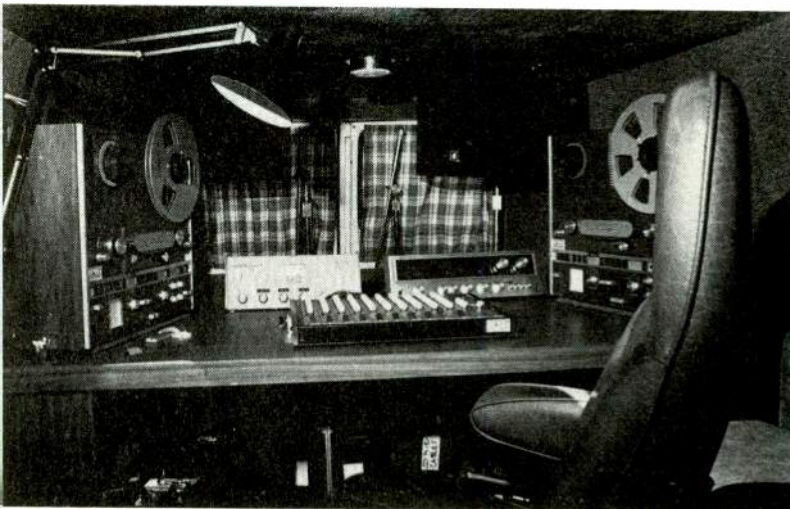
Operator position in concert van built by KPBS has multi-channel console on table, tape recorders left and right. Walls and ceiling have sound absorbing cover to improve acoustics for accurate monitoring
