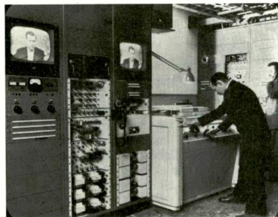
CBS engineer adjusts Ampex VTR during the first tape broadcast in November, 1956. All three networks adopted videotape over the next few months
