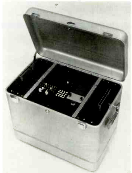
Completed PRB-II weighs 45 pounds, is easily carried into field and set up to supply emergency communications. Pushbuttons control microprocessor
