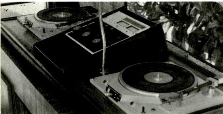
Operating position in field production van has two turntables for recorded program inserts, multi-channel mixer, and UHF radio for taking program to studio
