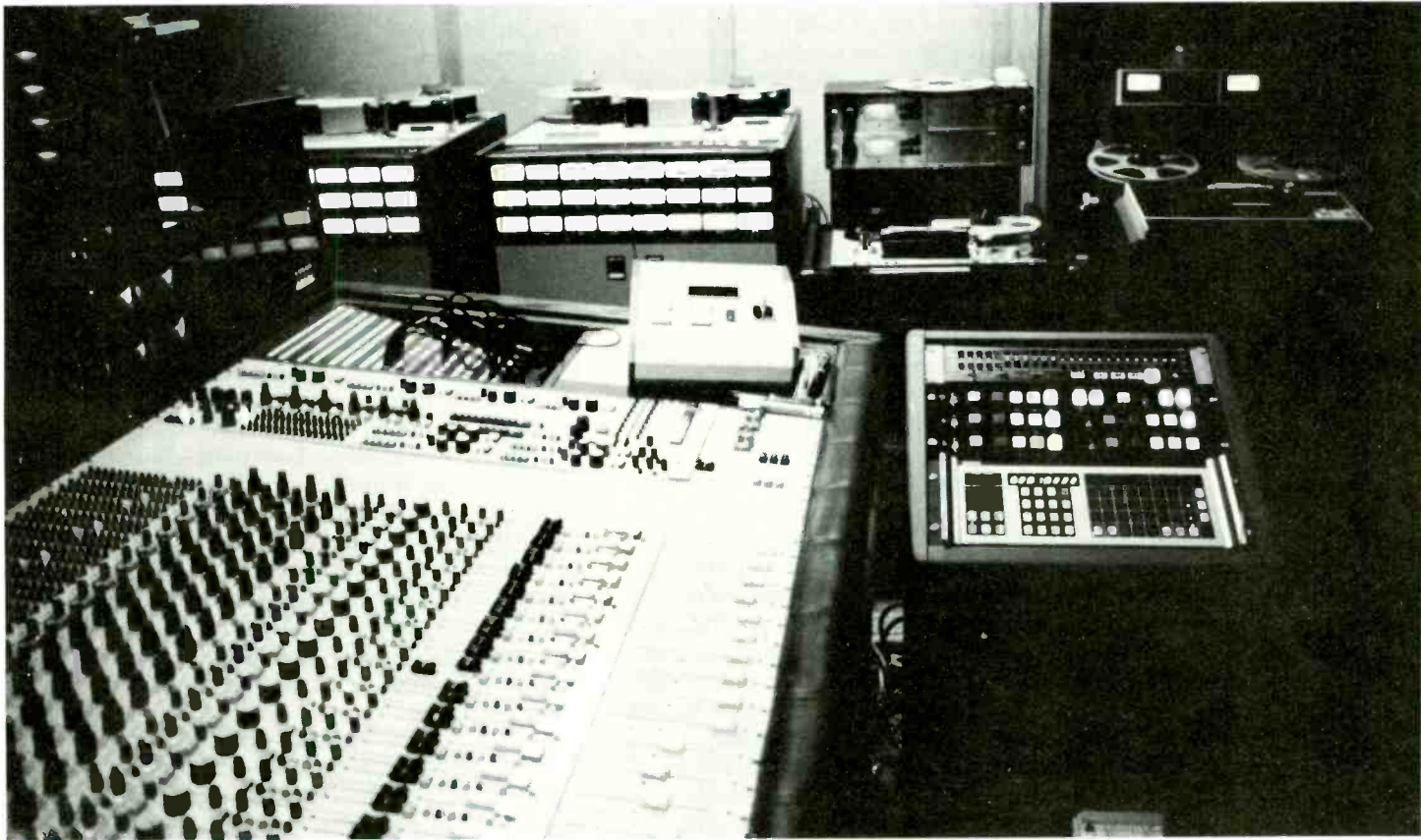
View of Regent Sound Studio's "full up" audio editing system. The "brain" of the system is the MQS-100 synchronizer housed in the console (center-right) which also contains remote controls for the various Ampex audio machines (background)
