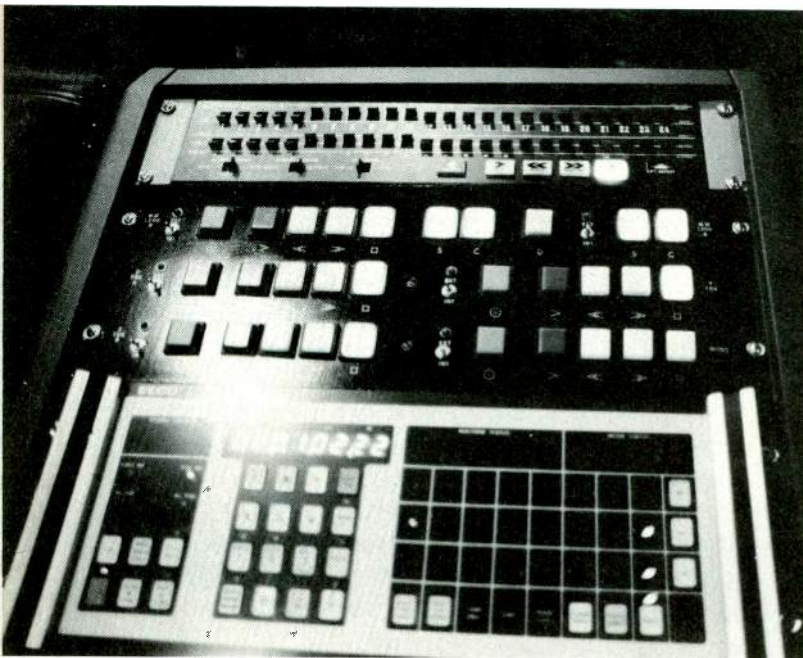
Close up of Regent Sound Studio's machine control editing console. Completely accurate sound to video editing is possible with this system. Effected tracks are switch selectable (top). Machine control panel (middle) is custom built, and MQS-100 (bottom) provides intelligence
