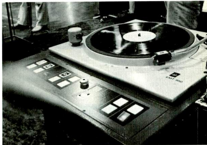
Important among factors taking broadcast quality to new, higher levels are the new electronic-control turntables, of which the EMT 950 (sold by Gotham Audio in the U.S.) is one. Flutter is nearly non-existent; noise is an order of magnitude lower than on many earlier tables
