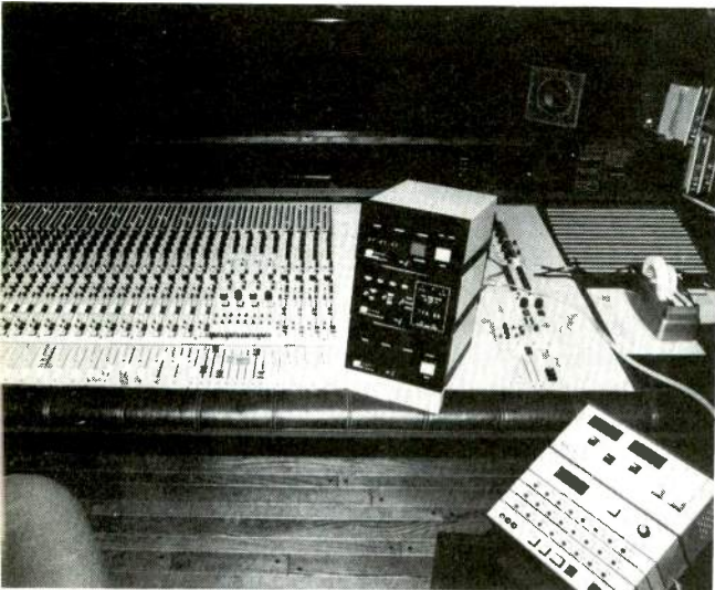
Soundmixers' MCI console with btx SMPTE components stacked. Top to bottom, the 4100 TC generator, the 4500 TC synchronizer, and the 4200 TC digital display
