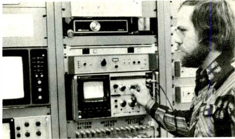
John Bowen, Rockford Cablevision engineer, looks at oscillator signals from various terminals on spectrum analyzer
