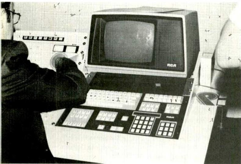
Dialogue with operator of the AE6000 and other editing data is displayed on CRT. Dual mini floppy disc is main mass storage facility
