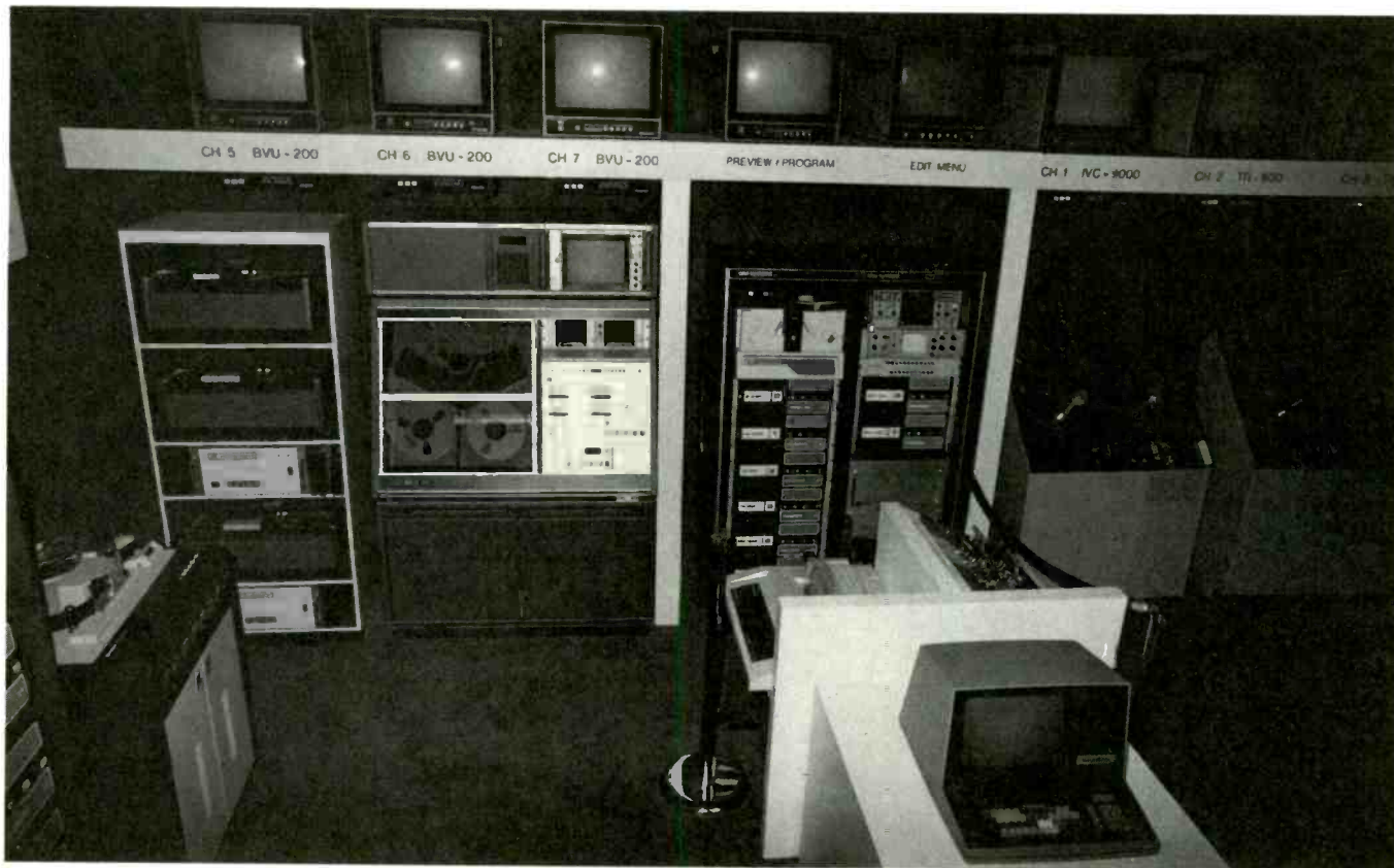
The use of microprocessors as part of intelligent interfaces was pioneered by CMX to make multi-machine, multi-format editing systems possible. The CMX 340X shown above is interfaced to three BVU VCRs, an IVC-9000 Helical scan 2-inch VTR, two quad TR-600s, and a Grass Valley Switcher. Dedicated interfaces are housed in the rack located in the middle rear of the picture
