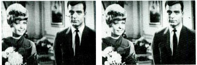
SMPTE standard slide as input (left) appears to be nearly perfectly reproduced (right) by 1/2 frame (one field) system when missing field is replaced by repeating first stored field.
