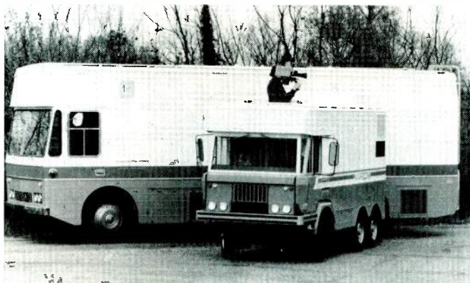
Marconi introduced the mini-mobile. It can be equipped with two small cameras, a VTR, video mixer, audio mixer, sync generators, monitors, test equipment and microwave link plus a power generator.
