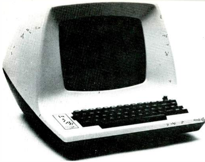
Lear-Seigler's "Glass Teletype"; model ADM-3 Video Display Terminal, marketed as a low-cost kit and sold over-the-counter in a number of retail computer stores in the major metropolitan areas.
