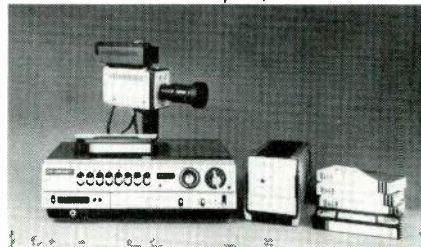
JVC's new Vidstar VHS™ system consists of: 2-hour videocassette recorder/player; the Vidstar camera, Model CG-3300U (shown here with 6:1 zoom lens and electronics viewfinder) and accompanying color camera adapter; and videocassettes with playing time of 2 hours, 1 hour and 1/2-hour.
