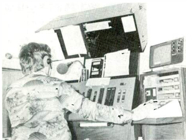
A third kind of radio automation is the IGM Mark VII which assists dj by putting music on push-button call-up, either singly or in pre-set sequences of almost any length. Operator can set up long program, interrupt or change at any time. This installation is at KTNT, Tacoma, WA.
