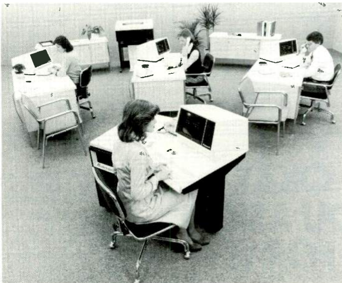
Automation Electronics (right) uses Honeywell computer for system with capability for combined traffic/billing and program switching; station can start with one, add other later. Photo emphasizes use of multiple inputs.
