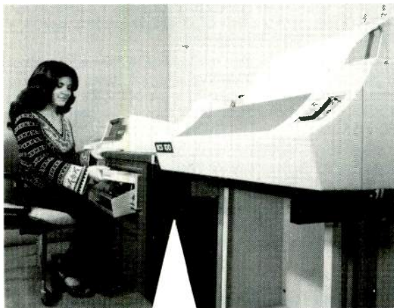
The Kaman Sciences' BCS-100 (above) represents another popular traffic/billing plan. System uses a large capacity central computer, plus mini-computer power at station. Interface to program automation is fully developed, in wide use.
