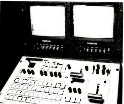
This Shintron switcher was one of many new small production switchers for vans and small studio operations.
