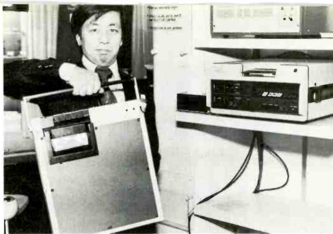
The NEC TTR-7 cartridge one-inch (battery) recorder weighs less than 30 lbs. TTR-5 A-C unit on shelf.
