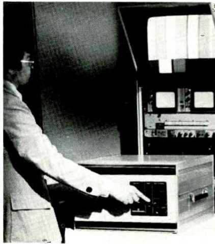
Digital Noise Reducer from Thomson-CSF provided remarkable improvement (9 or 12 dB) to noisy video.
