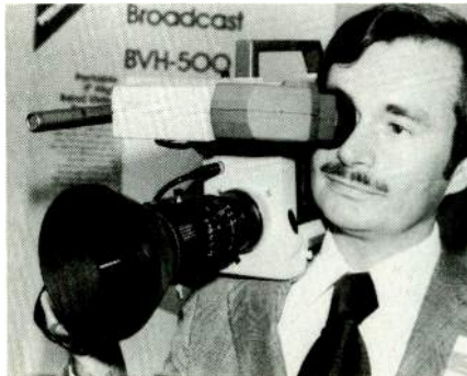
New Sony BVP-200 two-tube ENG camera.
