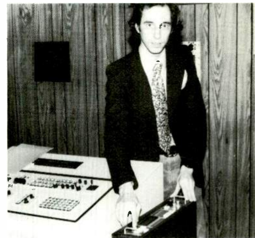
Steve Rutt displayed his $6800 Video Repositioner, the 1080. The device will "reposition new video" anywhere within the raster.
