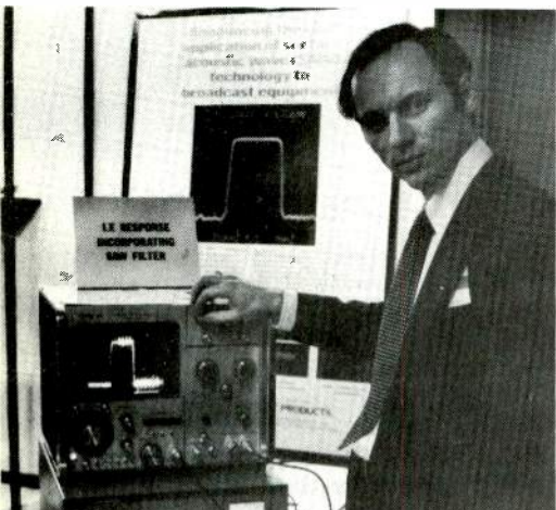
Sharp response of SAW filter shown by EMCEE.
