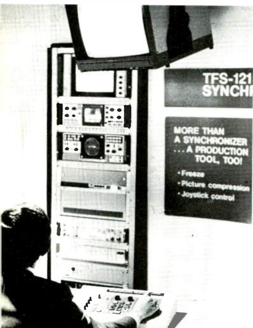
Frame synchronizers, like this TFS-121 from RCA, turned a lot of broadcasters on to the idea of special effects produced in the digital domain.
