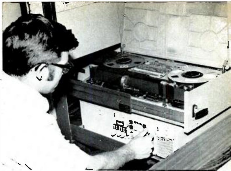
RCA's miniaturized quadruplex video tape recorder, the TPR-10, is shown in an outside broadcast van of Videomobile Systems, a Hollywood teleproduction company.
