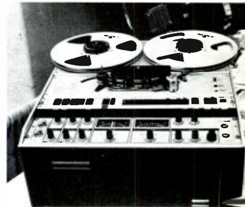
Ferrograph Studio 8 has modular electronics (very general), interchangeable head blocks.
