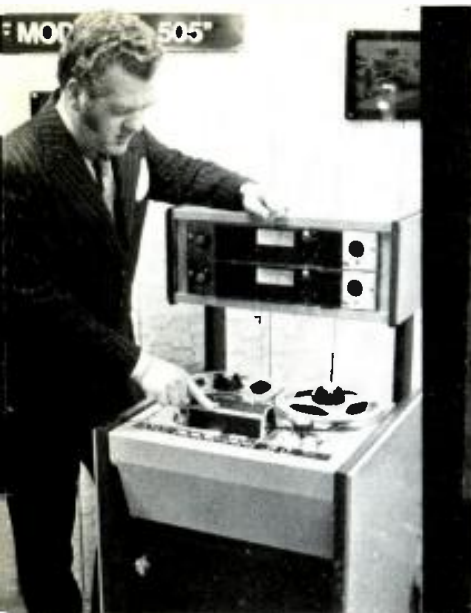
Electrosound 505, seen here at '74 NAB, has optional third reel to ease editing.
