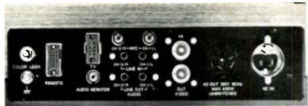
Fig. 4. Back of VO-2850 showing remote control receptacle.
