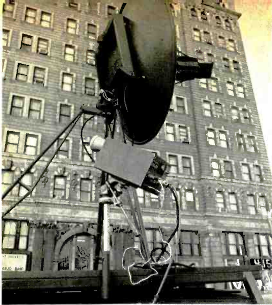
If there is a direct line between the camera and the van, the signal can be sent via RF (13 GHz) to the van for further microwave relay. Small unit with cone antenna aimed at building window is Microwave Associates MA-13P unit. Dish antenna is from Nurad.
