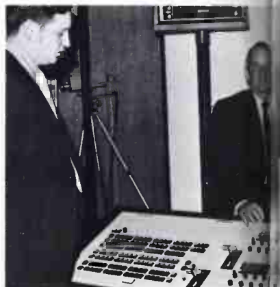
Visual's switcher permitted keyed inserts non-sync remotes while locked to station.
