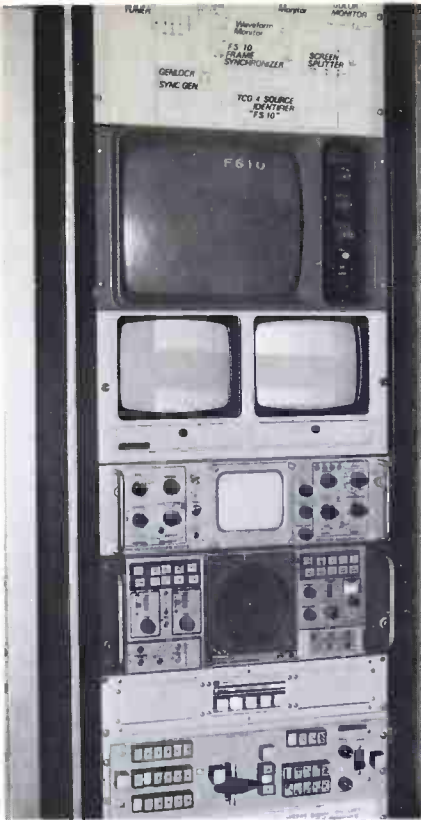
Super TBC from NEC/TeleMation locks any remote to station sync in one frame.
