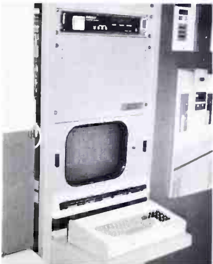
Central Dynamics' new APC610/200 (above) automates both traffic and switching; APC610/100 (below) handles technical operations only.
