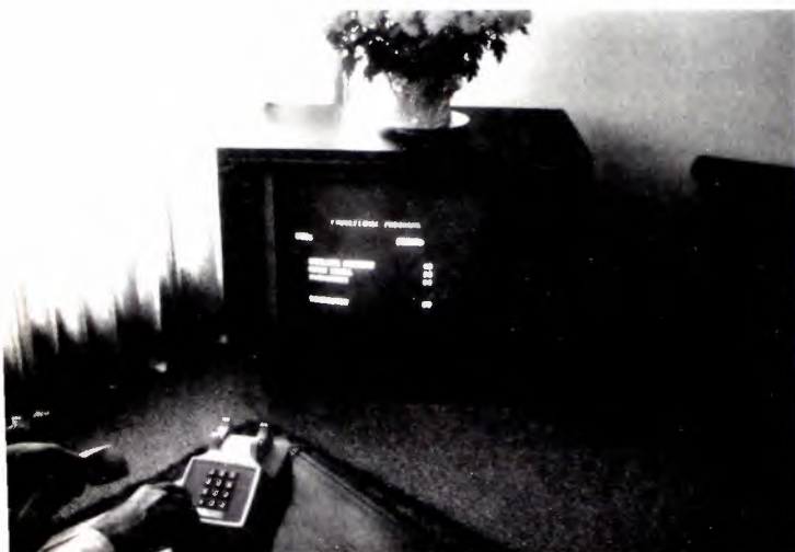
Mitre's TICCIT system can use a Touchtone telephone to feed back information to a cable TV headend.
