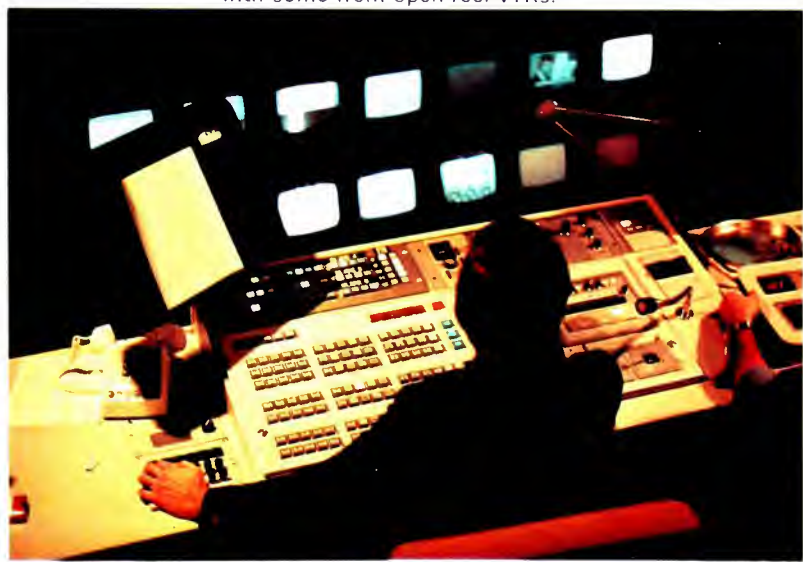
A main control position at WGR-TV, with large studio window facing operator, switcher under his right hand, studio monitors above window, monitors for other inputs below window, operation monitors at far left. Each studio has its own control room.
