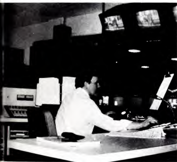
Looking over shoulder of program director Ernie Rouert at push-button panel of sub-control switcher (RCA TS-51) which receives inputs from studios, lines, VTRs etc., and routes them as required. Vidifont special-effects generator, and chroma keyer are also at position.
